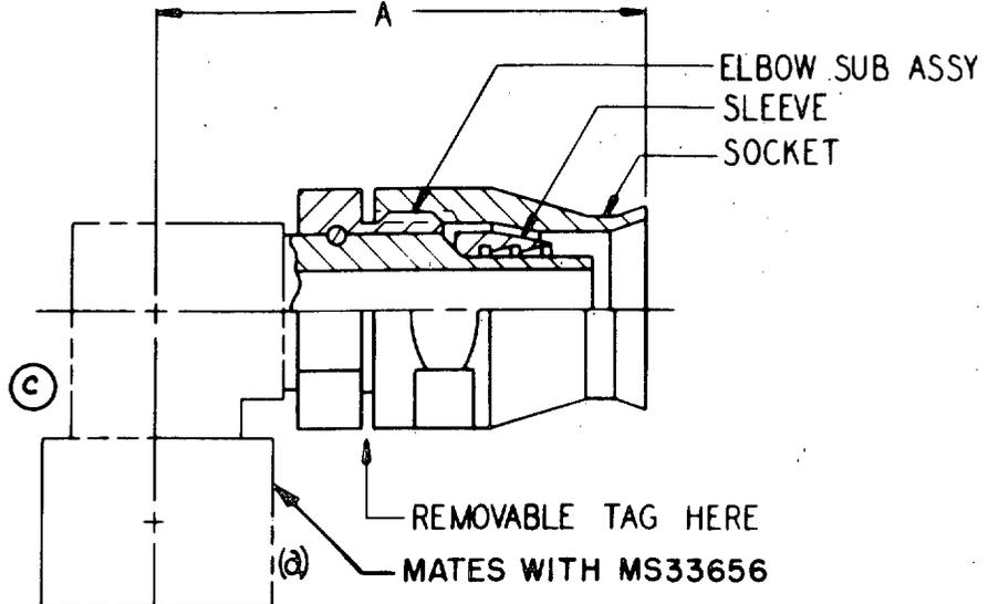
(C) "A" IS THE DIMENSION BETWEEN THE HOSE END OF THE SOCKET AND THE CENTERLINE OF THE INSERT WHEN THE SOCKET IS ASSEMBLED ON THE NIPPLE.
