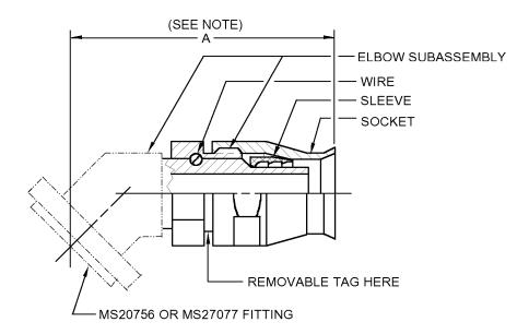
NOTE: A is the dimension between the hose end of the socket and the free end of the insert at its centerline when the socket is assembled on the elbow subassembly.
