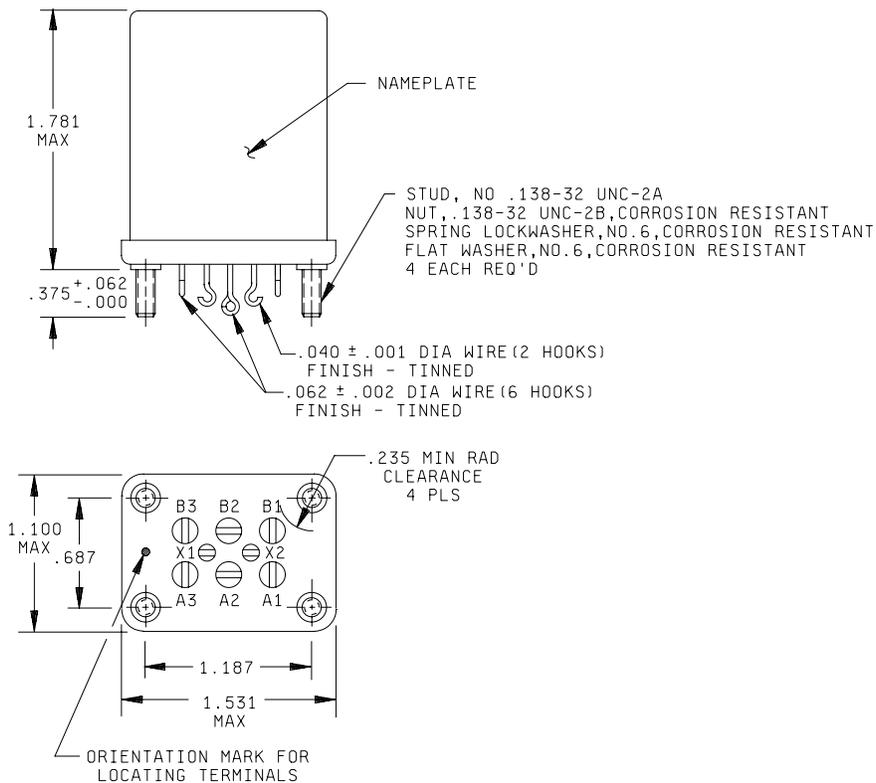
FIGURE 1. Dimensions and configurations.
