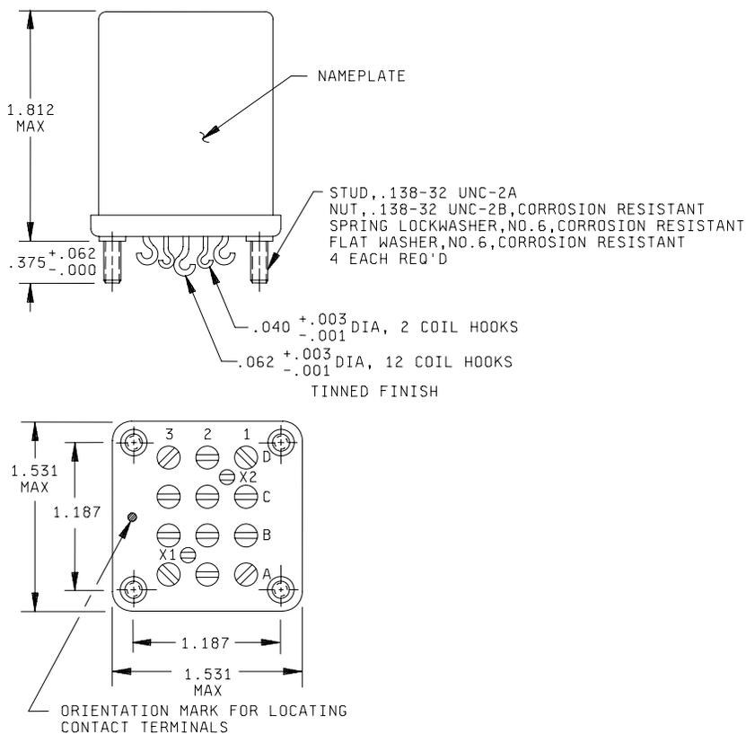
FIGURE 1. Dimensions and configurations.
