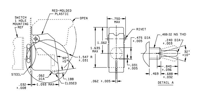
FIGURE 1. <u>Dimensions and configuration -1</u>.
