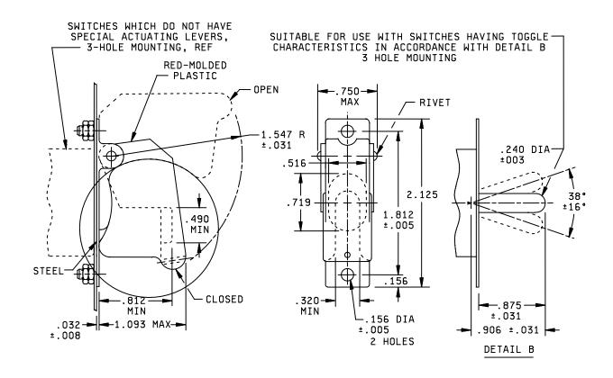
FIGURE 2. <u>Dimensions and configuration -2</u>.
