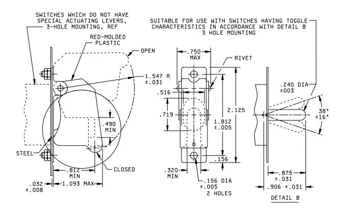
FIGURE 2. <u>Dimensions and configuration -2</u>.
