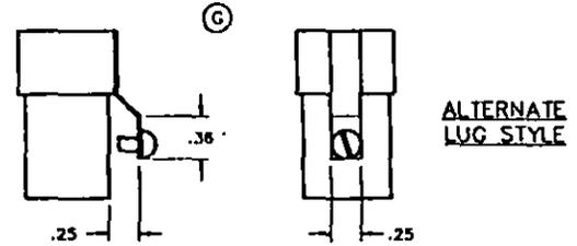
DIMENSIONS IN INCHES. UNLESS OTHERWISE SPECIFIED, TOLERANCES: DECIMALS ± .010; ANGLES ± 1°. PARTS UNDIMENSIONED ARE OPTIONAL WITH THE MANUFACTURER.
