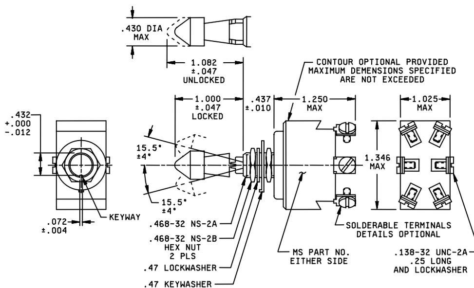
FIGURE 1 Dimensions and configurations
