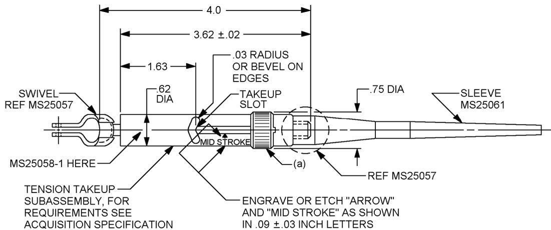
NOTE: Detent must be provided to hold locking ring in forward position against windows: 3 pounds, maximum 10 pounds disengaging force.
