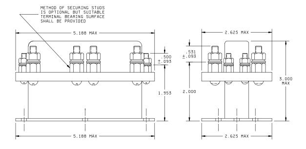
FIGURE 1. Dimensions and configuration.
