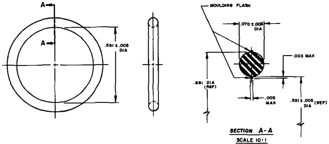
RINGS MAY BE OFF-REGISTER, DUE TO MOLD MISALIGNMENT, NOT TO EXCEED .003 INCH, PROVIDED ALL CROSS-SECTIONAL DIAMETERS, INCLUDING THE PROTRUSIONS (FLASH EXCLUDED) OF BOTH HALVES, WHERE APPLICABLE, SATISFY THE SPECIFIED CROSS-SECTION DIMENSION (.070 ± .003 DIA).
