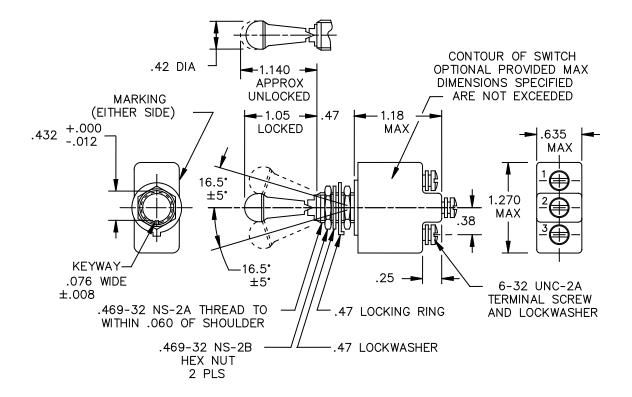
FIGURE1. Dimensions and configuration
