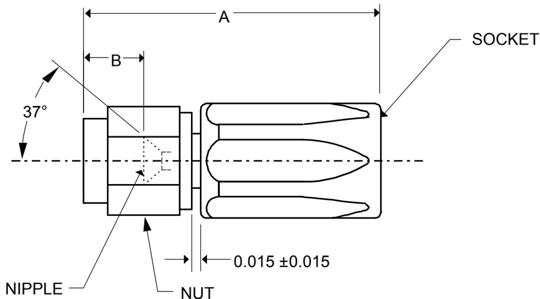
(NOTE: Nut must swivel freely after assembly)
