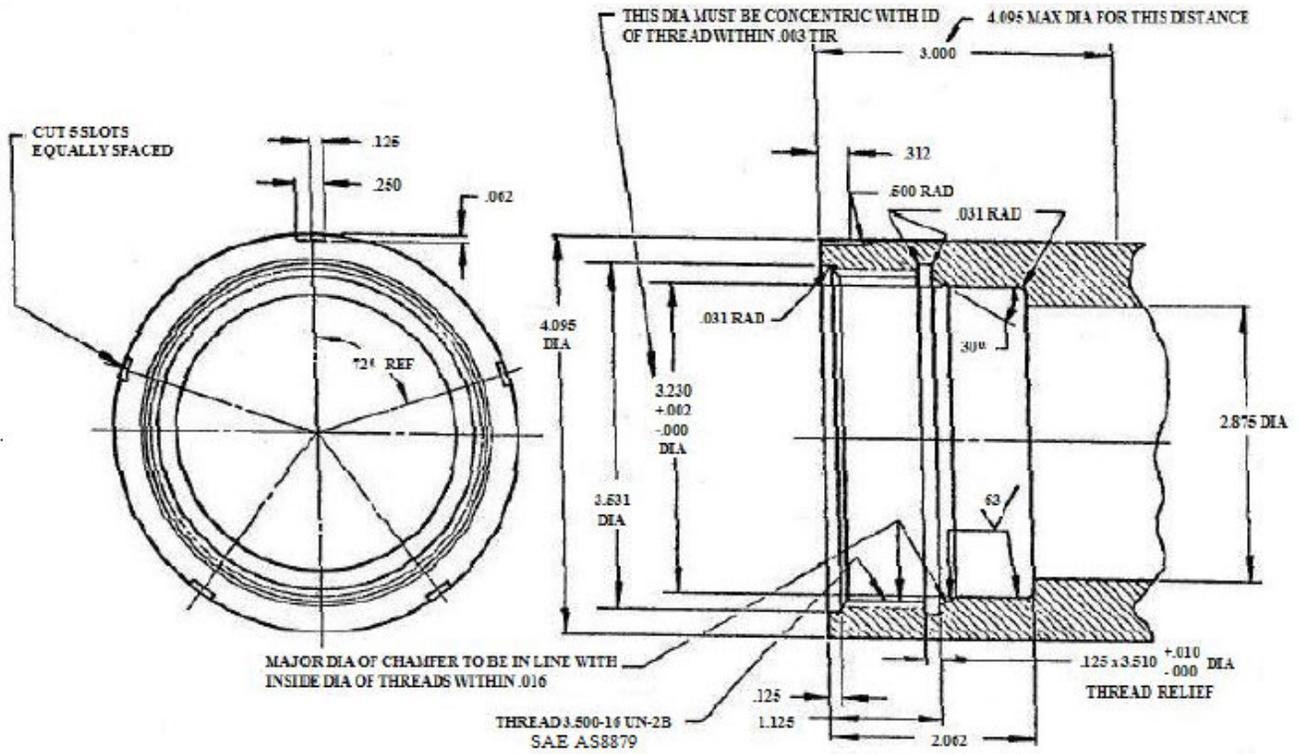
FIGURE 1. Nose, probe mast – type ma-2, flight pressure refueling nozzle, outline dimensions for.
