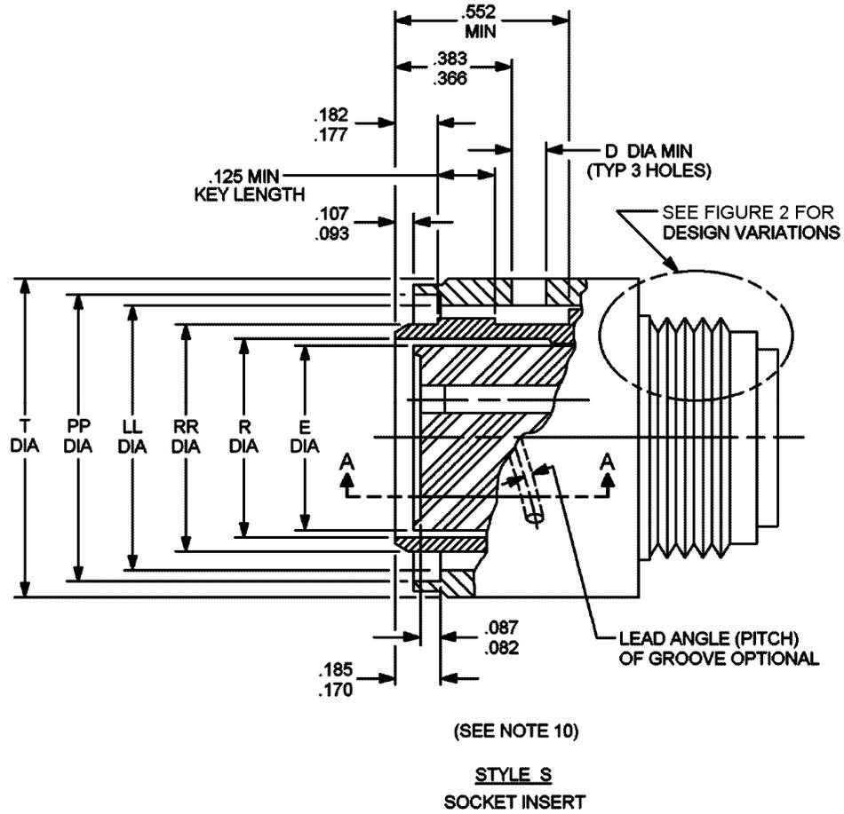
FIGURE 3. Plug, bayonet for classes F, G and R.
