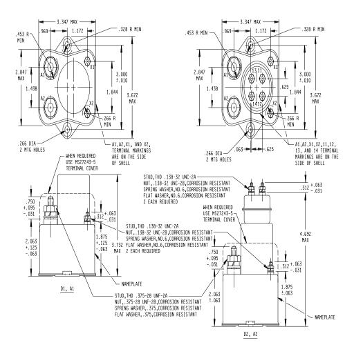
FIGURE 1. Dimensions and configurations.
