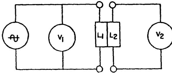
Equipment for 1 kHz and 10 kHz consists of General Radio Audio Oscillator and Power Amplifier type 1308-A, or equivalent and Model 400 vacuum tube voltmeter, or equivalent.
