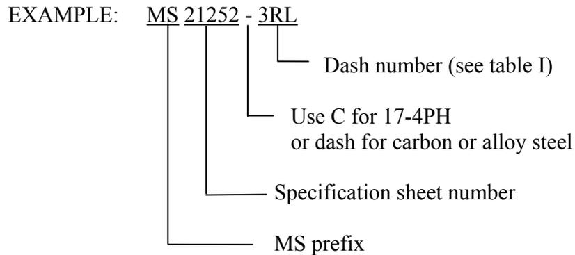
MS21252C3LS Indicates - Clevis end, 17-4PH, 0.1900 (#10)-32 left hand thread, short.
