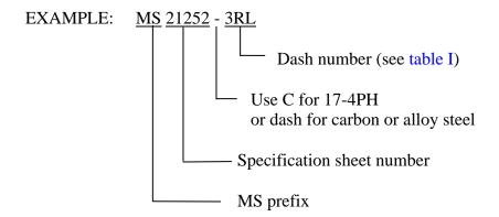
MS21252C3LS Indicates - Clevis end, 17-4PH, 0.1900 (#10)-32 left hand thread, short. MS21252-3RL Indicates - Clevis end, steel, 0.1900 (#10)-32 right hand thread, long.
