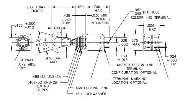
FIGURE 1. <u>Dimensions and configuration</u>.
