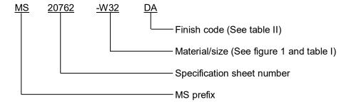
PIN example: MS20762-D32DA indicates a 2-inch 7075 aluminum elbow with chemical conversion coating in accordance with MIL-DTL-5541 type II, class 3.
