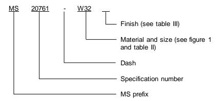
Example of PIN: MS20761-W32 is a 45° elbow, 7075 aluminum alloy, 2.000 inch (50.80 mm) tube diameter, and 2.750 (69.85 mm) flange, anodize in accordance with MIL-A-8625, type II dyed brown.
