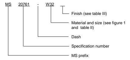
Example of PIN: MS20761-W32 is a 45° elbow, 7075 aluminum alloy, 2.000 inch (50.80 mm) tube diameter, and 2.750 (69.85 mm) flange, anodize in accordance with MIL-A-8625, type II dyed brown.
