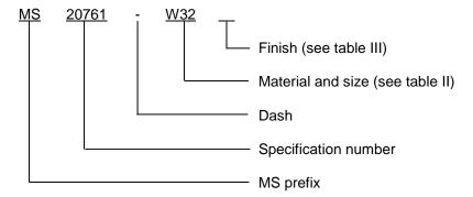
Example of PIN: MS20761-W32 is a 45° elbow, 7075 aluminum alloy, 2.000 inch (50.80 mm) tube diameter, and 2.750 (69.85 mm) flange, "blank" code for AI is "anodize in accordance with MIL-A-8625, type II dyed brown.
