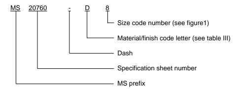
PIN example: MS20760-D8 indicates a flange to hose adapter .500 inch (12.70 mm) flange to a .750 inch (19.05 mm) thread, aluminum alloy 2014-T4 anodized light blue.
