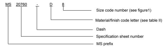
PIN example: MS20760-D8 indicates a flange to hose adapter .500 inch (12.70 mm) flange to a .750 inch (19.05 mm) thread, aluminum alloy 2014-T4 anodized light blue.
