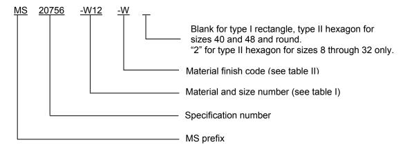
MS20756-W12W indicates: Flange, .750 inch (19.05 mm) tube ID, aluminum anodized with NAVAIR TCP, type I rectangle.
