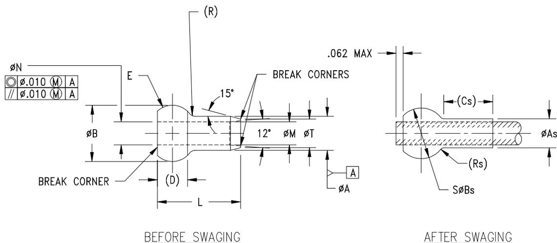
FIGURE 1. Ball end, wire rope, swaging, single shank.
