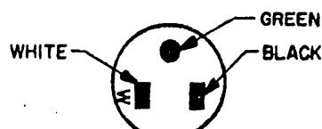
(B) PLUG CONNECTOR WIRING SEE REQUIREMENT 3
