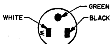
(B) PLUG CONNECTOR WIRING SEE REQUIREMENT 3
