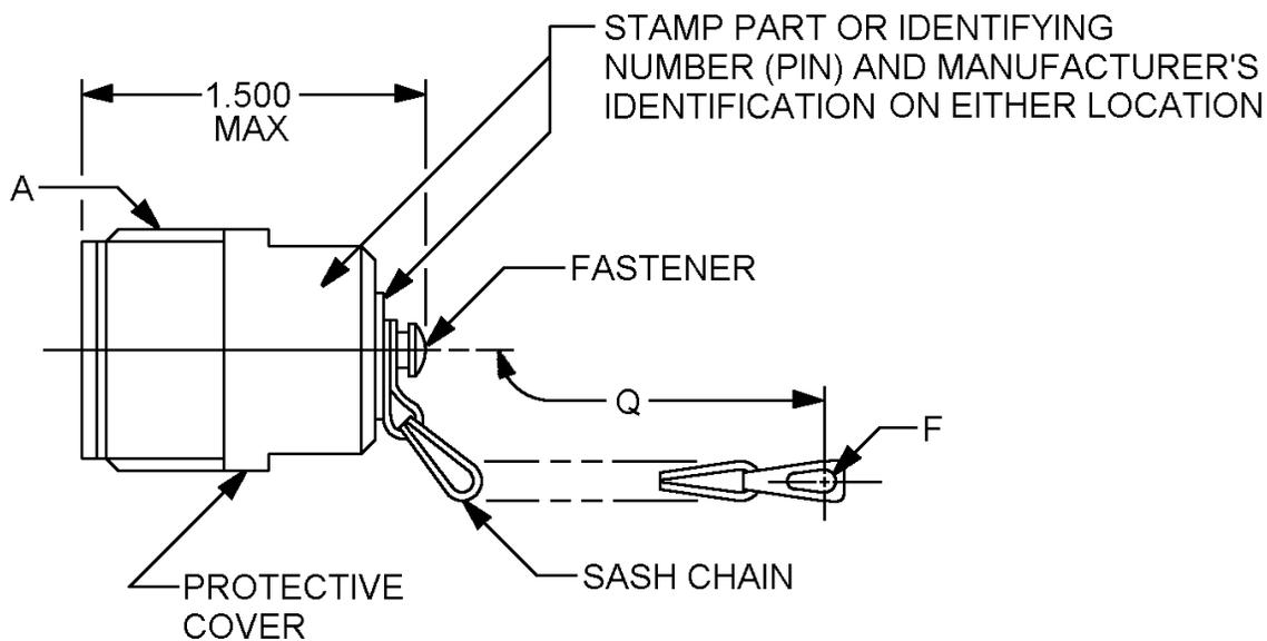
FIGURE 1. Dimensions and configuration.
