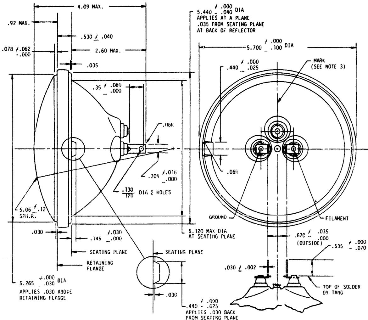
NOTE: INTERSECTION OF VERTICAL AND HORIZONTAL CENTERLINES THROUGH CONTACTS MUST FALL WITHIN .25 OF AXIS OF LAMP.
