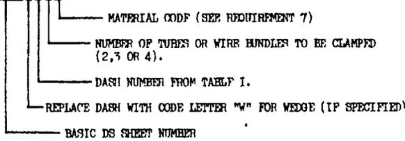
DS14272W223CF - INDICATES CLAMP, LOOP, CUSHIONED, ELONGATED, FOR 22mm Ø TUBING OR WIRE BUNDLES, 3 TUBES OR BUNDLES, CRES BAND MATERIAL WITH NITRILE CUSHION MATERIAL.
