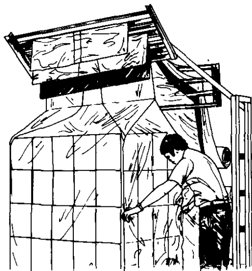
Figure 9.—Placing a shrink bag over a unitized load. (ML86 5124)
