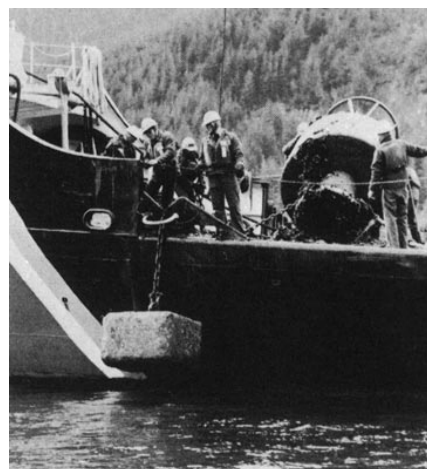
Figure 512. A sinker used to anchor a buoy.
