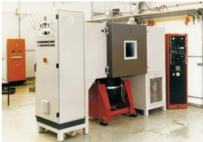
Figure 15-22: A controlled environmental chamber with vibration capability.
