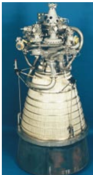
Figure 3-24: An engine with a large, regeneratively cooled nozzle.
