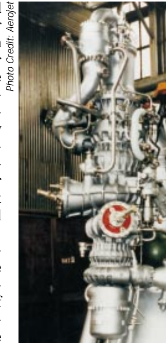
Figure 3-35: A single-shaft turbopump.
