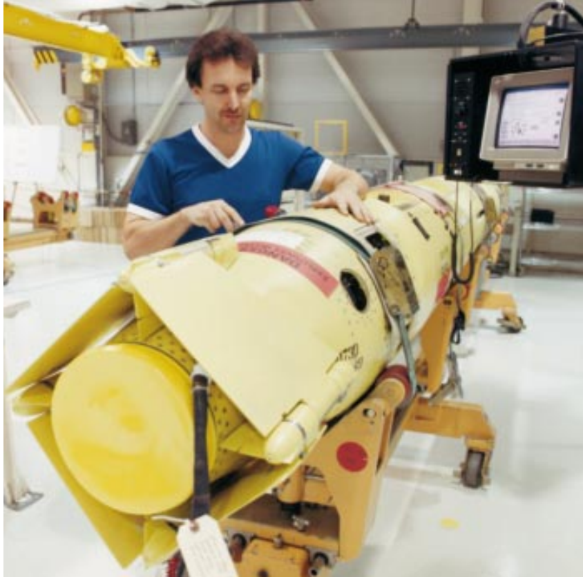
Figure 1-13: Modular jig supporting a cruise missile in final assembly.
