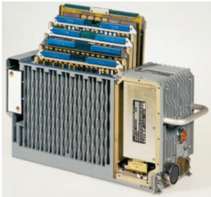
Figure 13-2: A ruggedized computer for fighters, which is similar to a missile or an UAV computer.
