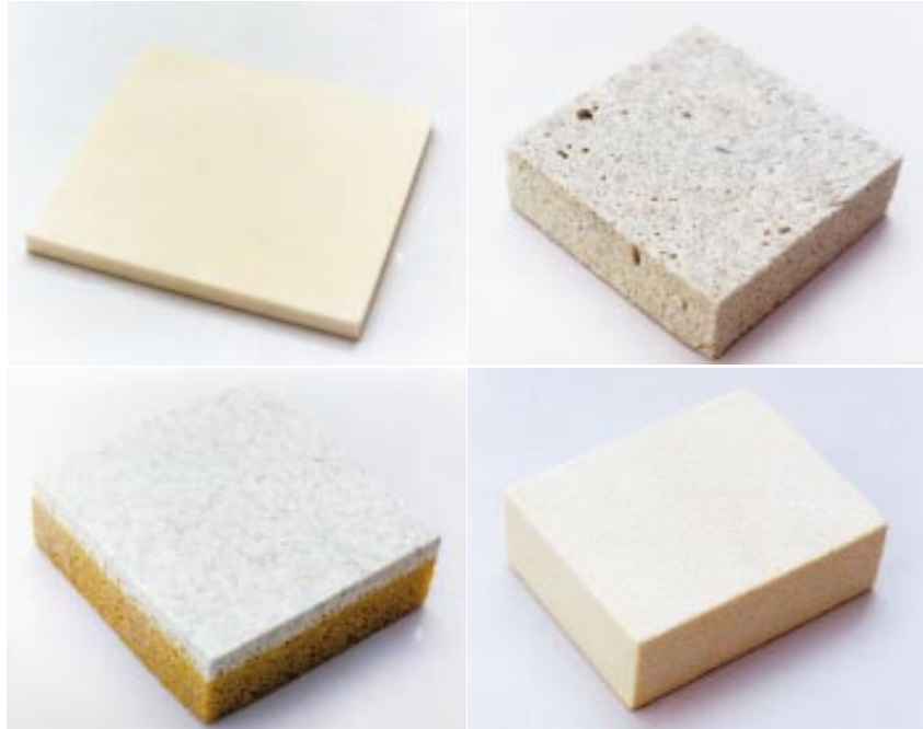
Figure 17-1: Four radar absorbing material foams, clockwise from upper left: low-dielectric foam (epoxy); lightweight lossy foam (urethane); thermoplastic foam (polytherimide); and sprayable lightweight foam (urethane).
