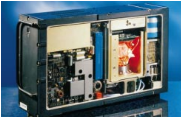
Figure 2-23: A guidance set using ring laser gyros.
