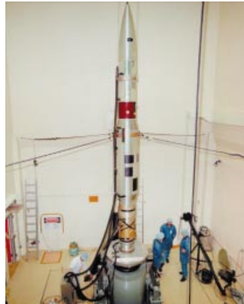
Figure 15-3: A missile vibration test facility and thruster.
