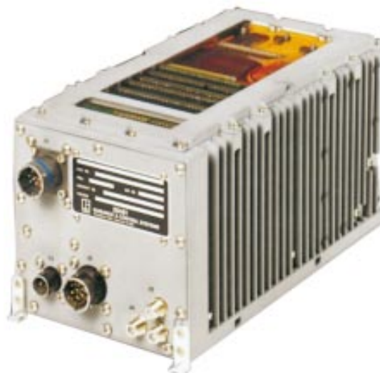
Figure 11-4: A complete guidance package based upon Global Positioning System receivers.
