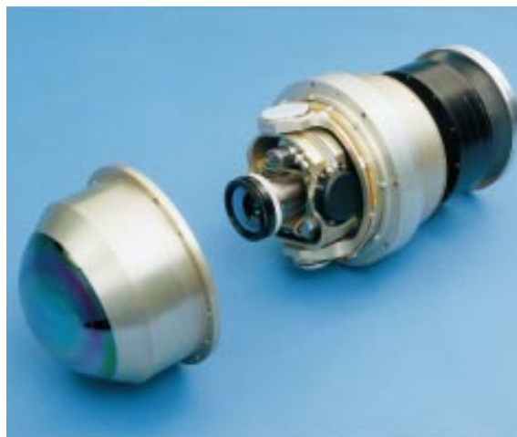
Figure 11-2: A gyro stabilized IR camera with its window.
