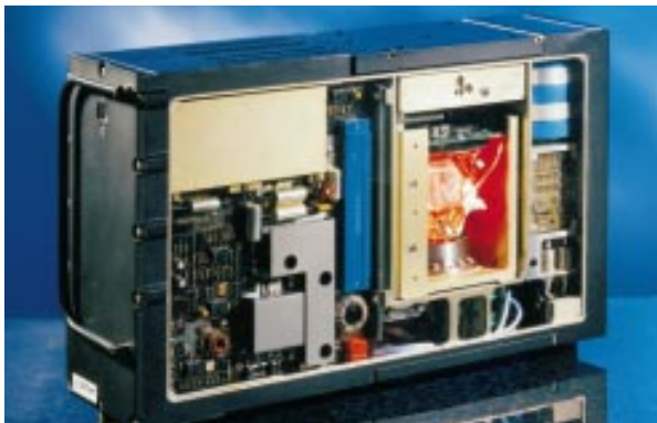
Figure 2-23: A guidance set using ring laser gyros.
