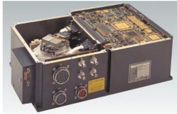
Figure 2-24: A guidance set using hemispheric resonating gyros.
