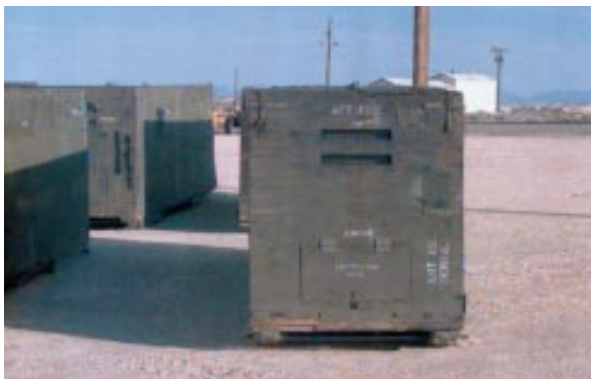
Figure 20-3: End view of a shipping container containing four Category II solid rocket motors.
