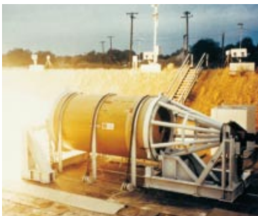
Figure 15-12: An outdoor, horizontal solid rocket motor test stand showing the dolly and frame holding the motor
