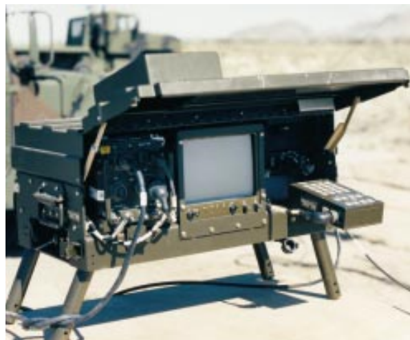
Figure 12-25: A portable video monitor for displaying video transmitted from an unmanned air vehicle.
