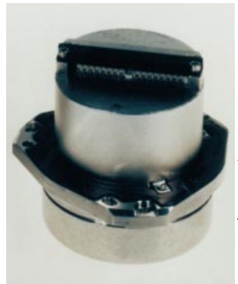
Figure 9-7: A DTG dynamically tuned spinning mass gyro.
