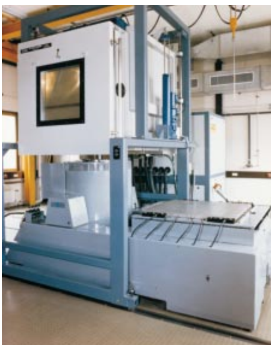
Figure 15-23: Another vibration and environmental test apparatus configuration.
