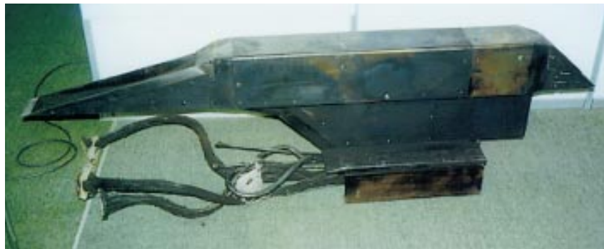
Figure 3-9: A developmental scramjet engine.
