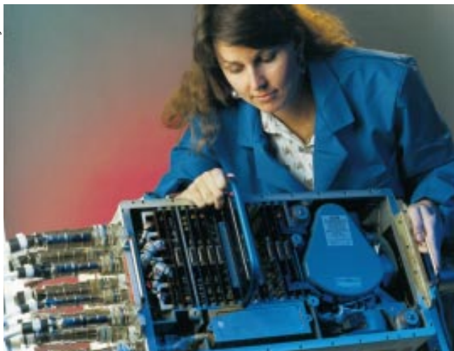
Figure 9-16: A strapdown IMU that contains three accelerometers and three ring laser gyros (in the end opposite the cables).
