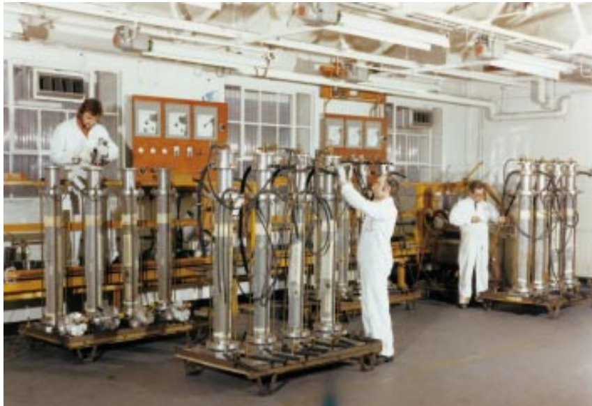
Figure 5-1: Tactical motors with cast-cure tooling attached.
