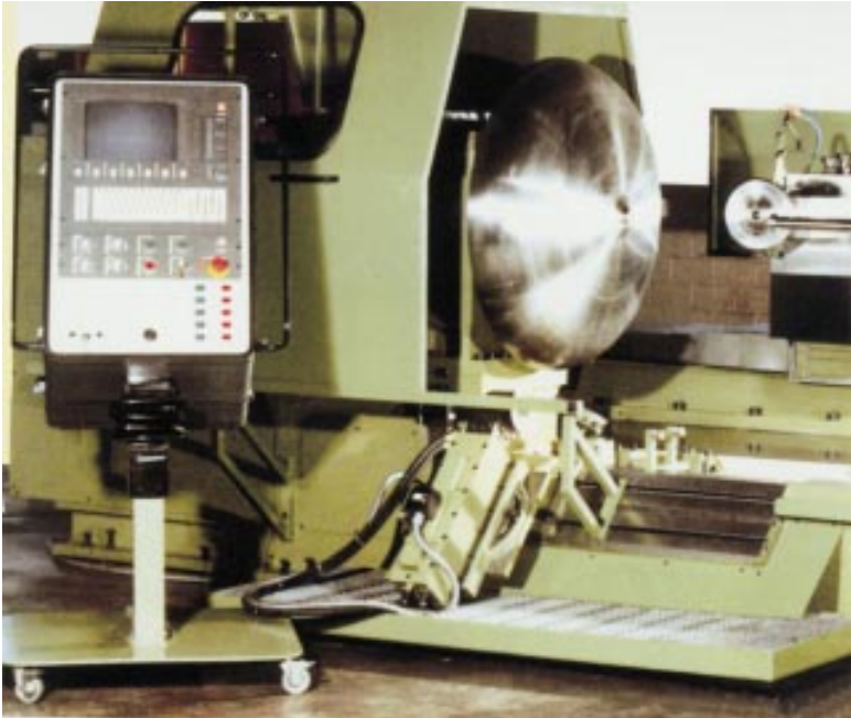
Figure 3-40: A flow-forming machine used to make end domes for propellant tanks.
