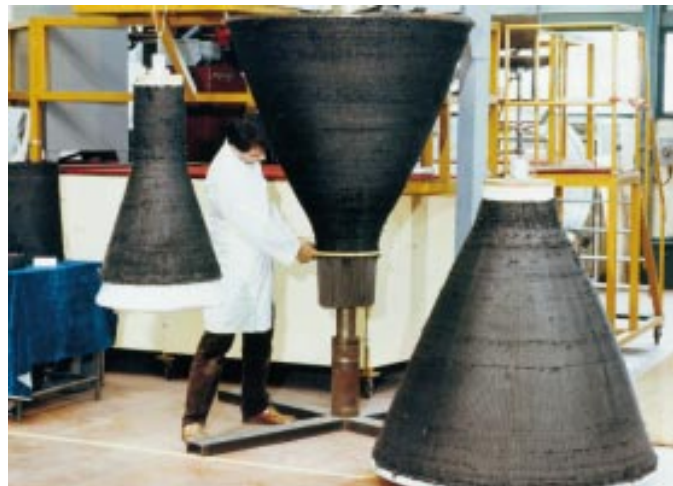
Figure 8-3: Preforms of rocket nozzle skirts.
