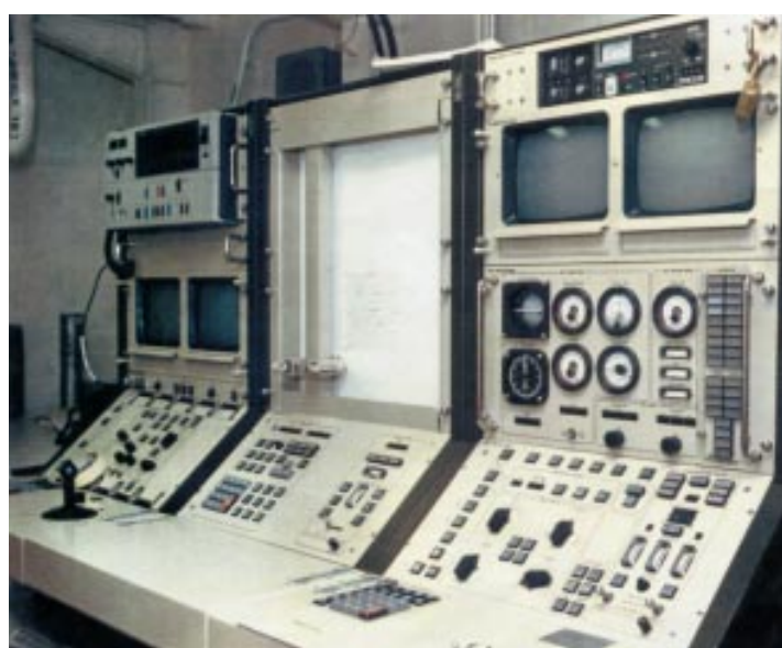
Figure 12-26: An integrated unmanned air vehicle control station.
