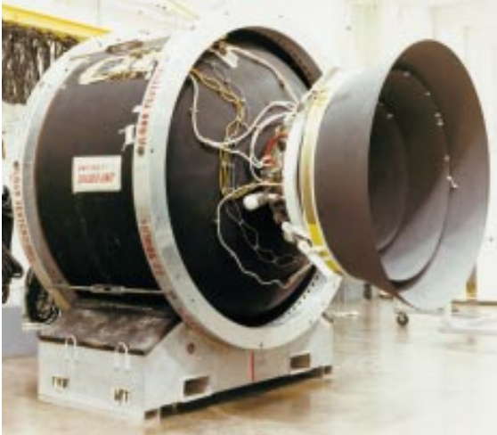
Figure 2-15: A solid rocket motor with an advanced, extendable nozzle skirt.
