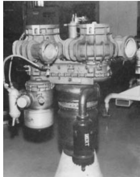
Figure 3-36: A multi-shaft turbopump assembly.
