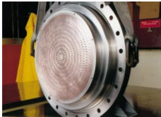
Figure 3-33: A liquid propellant injector plate.
