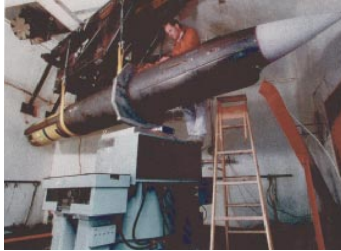
Figure 15-2: A thruster being prepared to vibration-test a missile.
