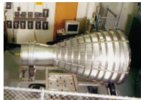
Figure 3-25: Side view of a regeneratively cooled nozzle.
