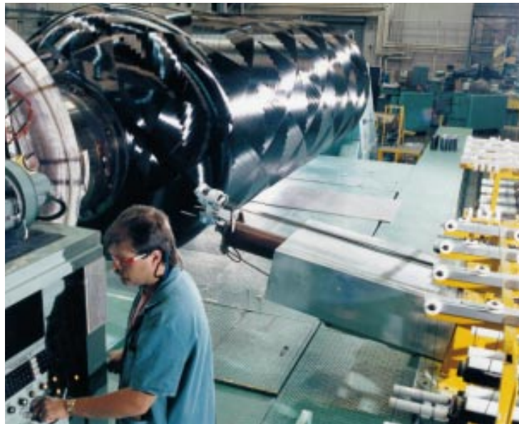
Figure 6-3: The filament winding machine with the multiple spools of fiber on the right.
