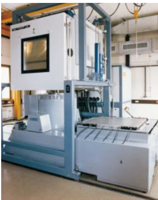
Figure 15-23: Another vibration and environmental test apparatus configuration.
