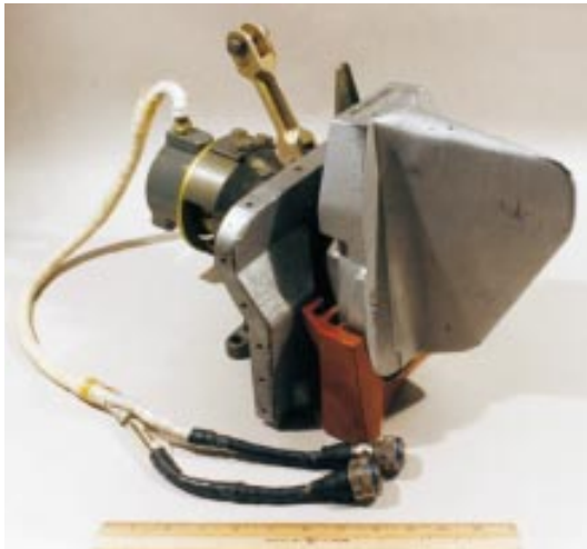
Figure 2-31: A jet vane for a liquid rocket.
