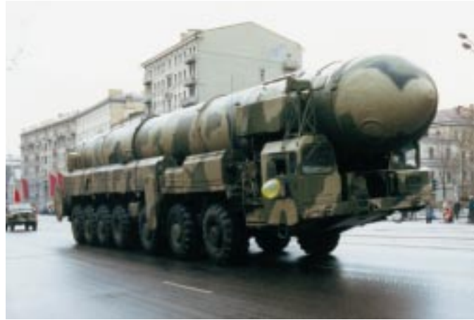
Figure 12-3: An ICBM transporter erector launcher with the missile in a launch canister.
