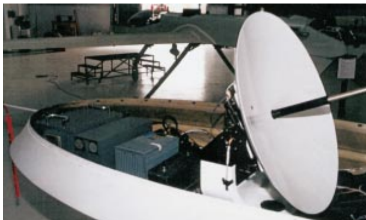
Figure 12-21: A SATCOM antenna installed in an unmanned air vehicle.
