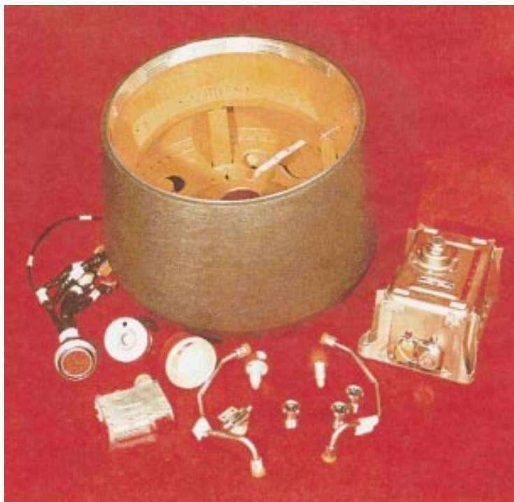
Figure 2-38: The aft end of an RV with the aft arming and fusing electronics box on the right.
