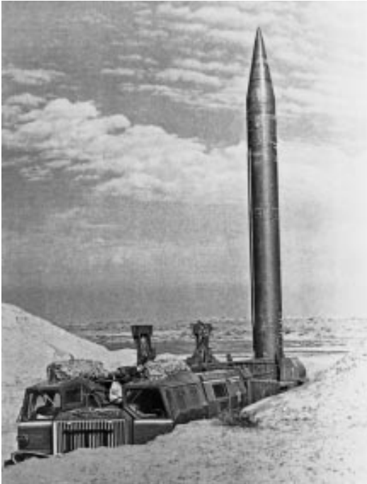
Figure 12-2: Transporter erector launcher with a short-range ballistic missile erected.
