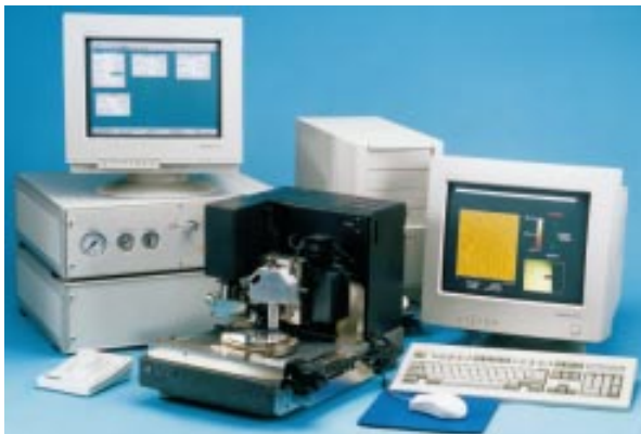
Figure 9-18: A profilometer system used for measuring mirrors.
