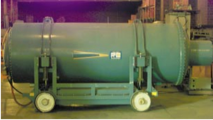
Figure 15-28: A 2.3MeV flash X-ray unit used for inspecting solid rocket motors.
