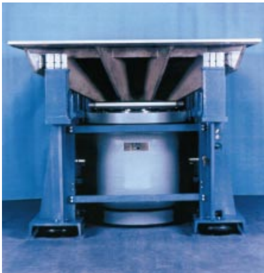
Figure 15-4: A thruster with an expanded head.
