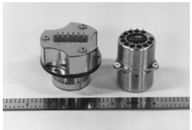
Figure 9-12: Two continuous output accelerometers, visually identical to those of Figure 9-5, rated at 100 g.
