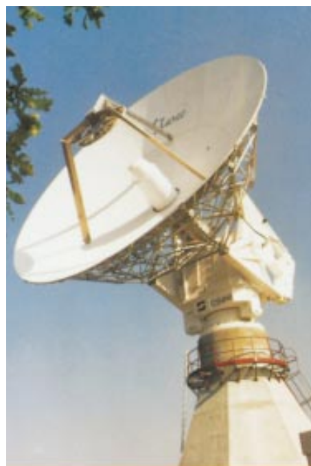
Figure 12-17: A typical, but large telemetry reception antenna.
