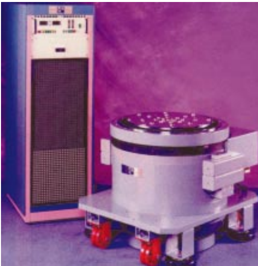
Figure 15-6: A power amplifier and its associated thruster.
