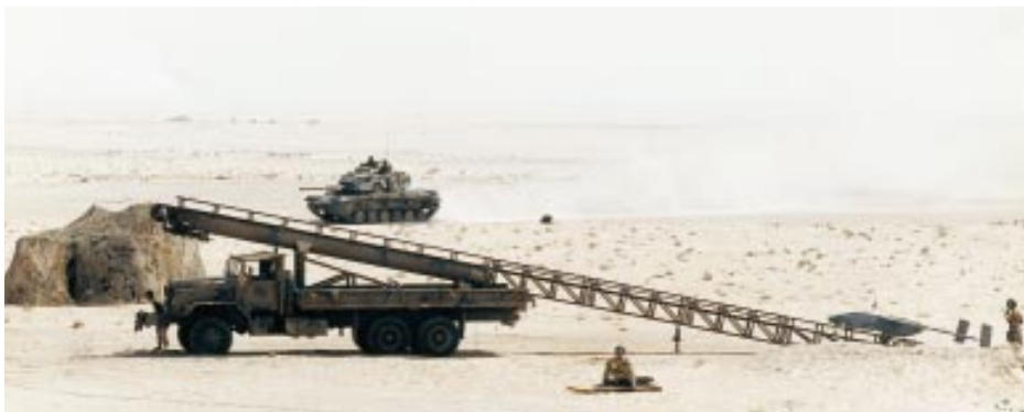
Figure 12-9: A pneumatic unmanned air vehicle launcher.
