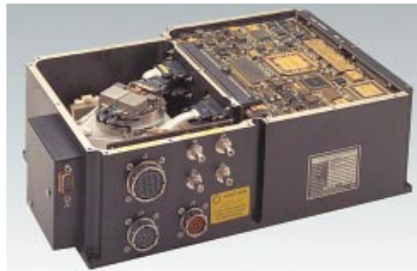
Figure 2-24: A guidance set using hemispheric resonating gyros.
