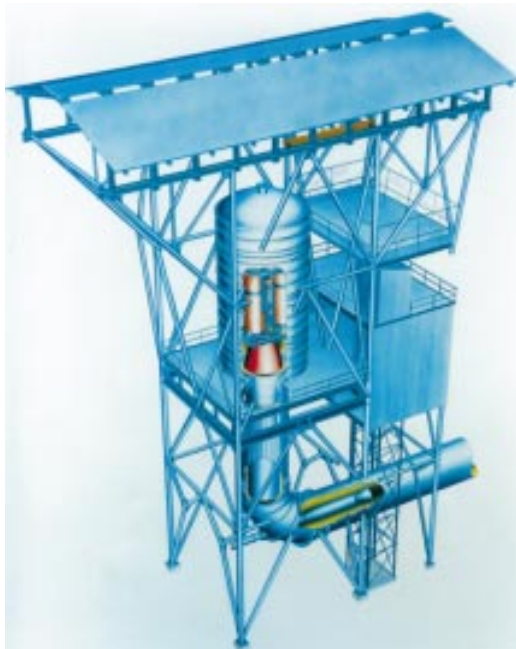
Figure 15-18: A different approach to an altitude test stand. The test object is shown in red inside the pressure vessel.
