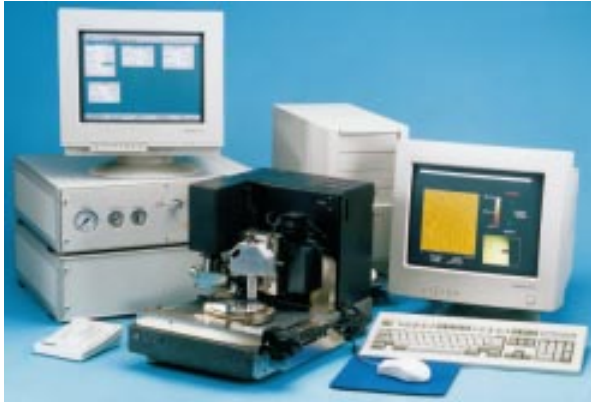
Figure 9-18: A profilometer system used for measuring mirrors.
