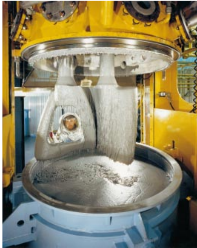
Figure 5-6: Open-blade configuration of a batch mixer.
