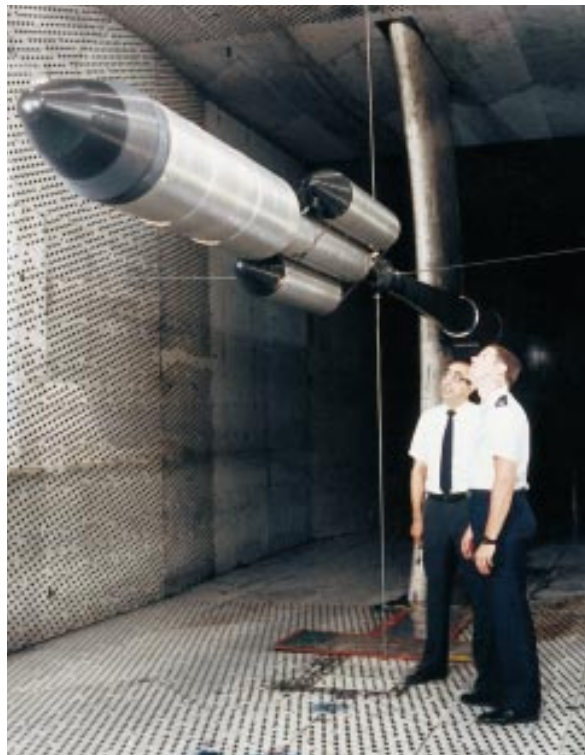
Figure 15-10: Test object under inspection in test section of a 5-meter transonic wind tunnel.
