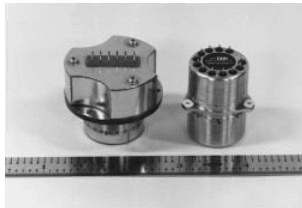
Figure 9-12: Two continuous output accelerometers, visually identical to those of Figure 9-5, rated at 100 g.
