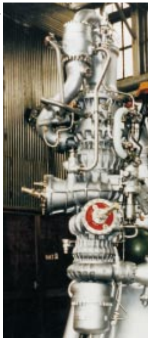
Figure 3-35: A single-shaft turbopump.
