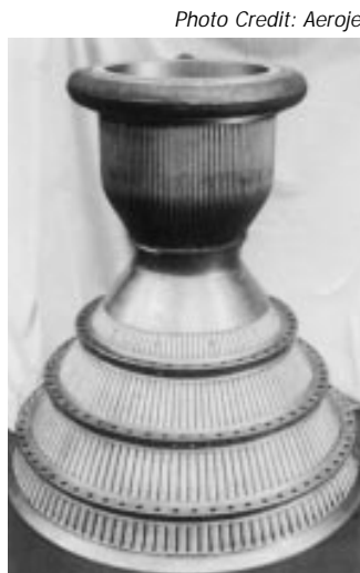
Figure 2-18: Combustion chamber and nozzle throat of a liquid propellant engine.
