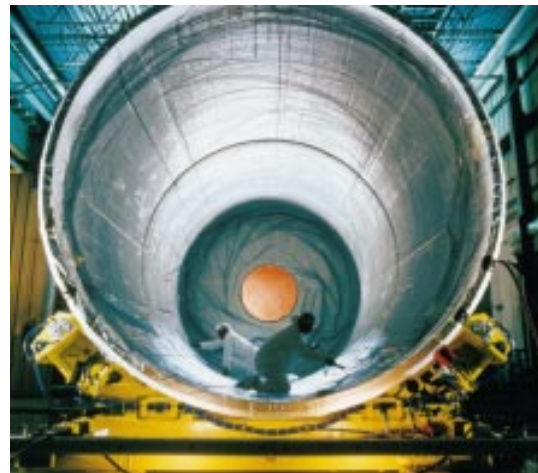
Figure 3-18: Installation of lining inside a motor case.
