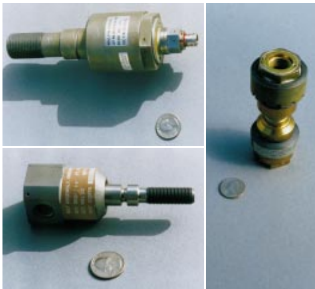
Figure 3-27: Three examples of explosive bolts. Notice the electrical connection on the top bolt, which detonates it.
