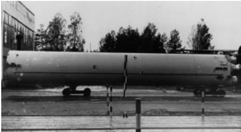
Figure 2-2: The first stage of a liquid-fueled ICBM.
