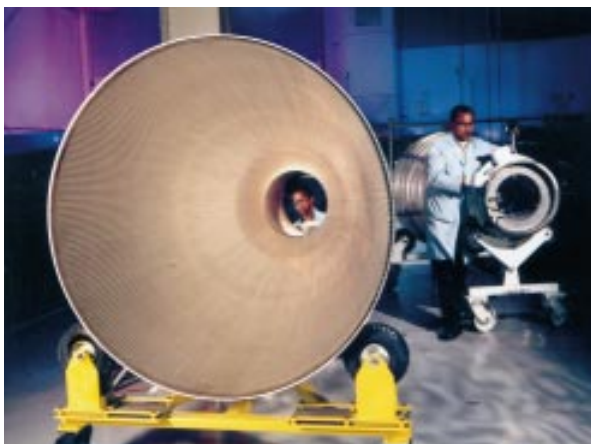
Figure 3-26: End views of regeneratively cooled nozzles.
