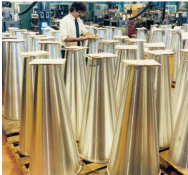
Figure 2-9: Modern RV mid-sections during manufacture.
