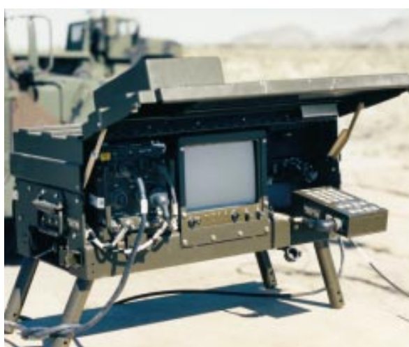
Figure 12-25: A portable video monitor for displaying video transmitted from an unmanned air vehicle.
