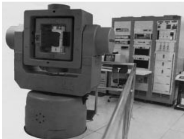
Figure 9-21: A three-axis rate table for testing IMUs or gyros.
