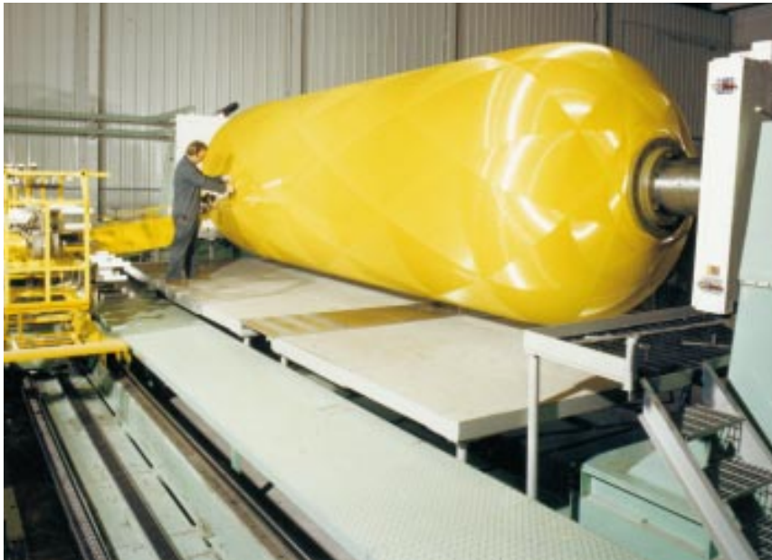
Figure 6-2: A large multi spindle filament winding machine.
