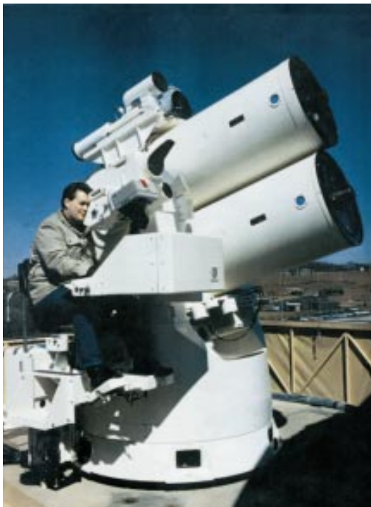
Figure 12-30: An optical missile tracking system.
