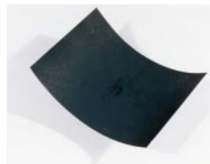
Figure 17-3: A sample of resistive card (R-card) made of metallized Kapton.
