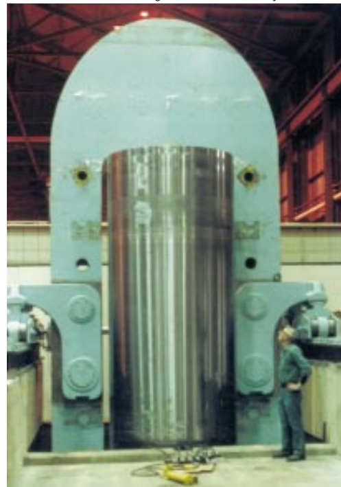
Figure 7-4: Side view of a large isostatic press.
