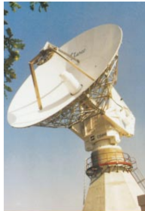
Figure 12-17: A typical, but large telemetry reception antenna.
