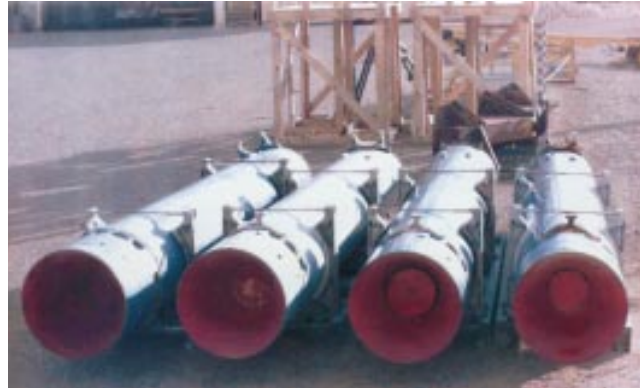
Figure 2-16: Solid rocket motors with total impulse close to the lower limit of Item 2 control.
