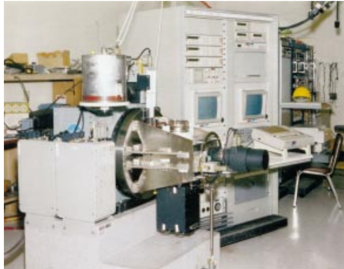
Figure 9-26: A dividing head with a temperature control chamber for testing an accelerometer inside the chamber.
