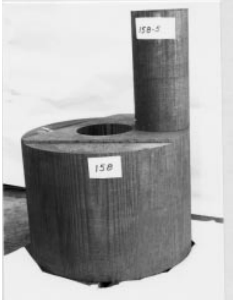
Figure 8-6: A block of carbon-carbon material ready to be machined into a rocket nozzle. The larger cylindrical block is about 70 cm in diameter.
