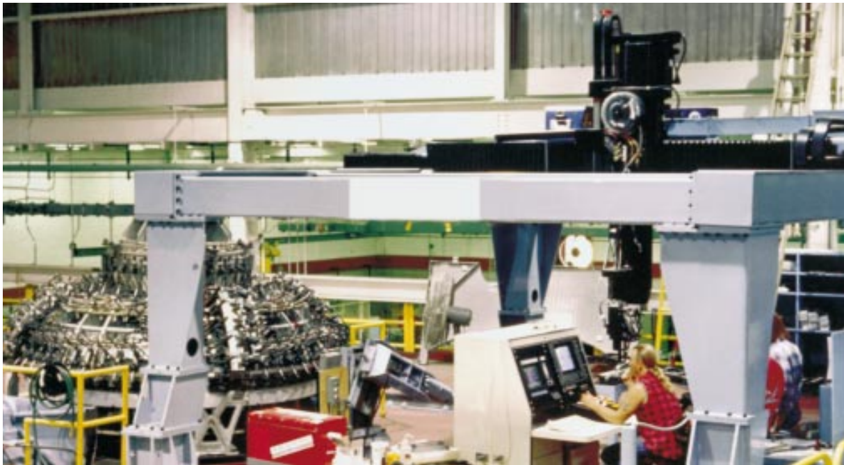
Figure 1-12: On the left, a very precise hydraulically adjustable welding fixture for a liquid propellant tank end dome; its seven-axis gantry robot welder is on the right.
