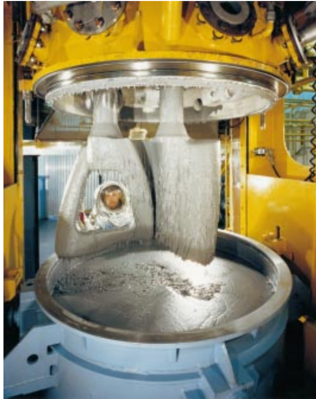
Figure 5-6: Open-blade configuration of a batch mixer.
