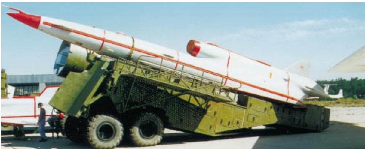
Figure 1-7: A jet powered reconnaissance UAV sitting on its launcher.
