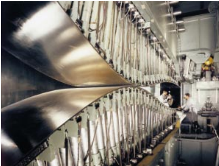
Figure 15-8: Exposed adjustable nozzle section of wind tunnel.
