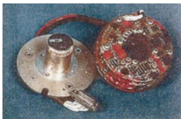
Figure 2-36: An RV SAFF system accelerometer with its associated electronics.
