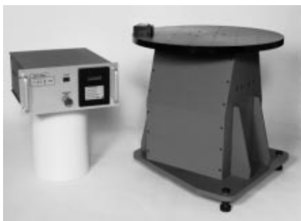
Figure 9-22: A typical rate table used for tuning gyros.
