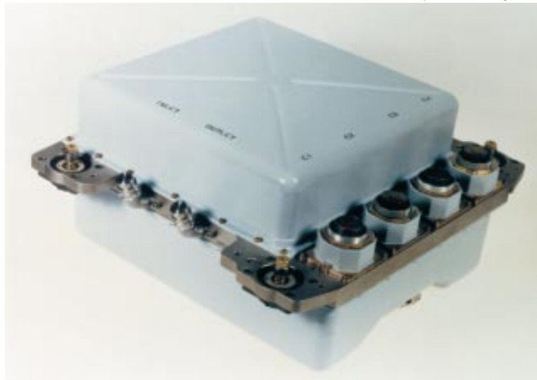
Figure 13-4: A radiation-hardened electronics assembly with liquid cooling.
