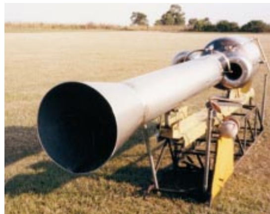
Figure 3-10: A modern pulsejet engine with a rearward-facing intake.
