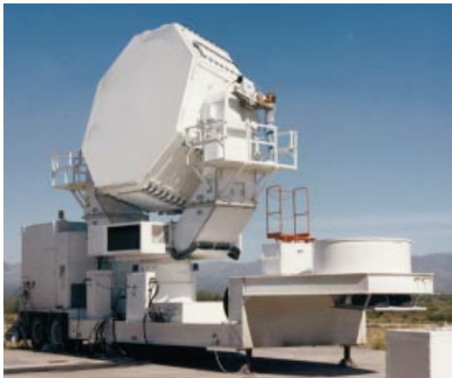
Figure 12-27: A mobile phased array missile tracking radar.
