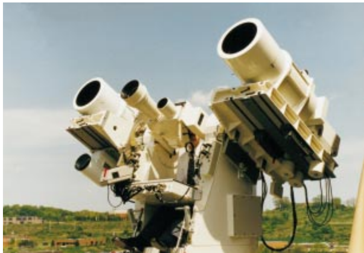
Figure 12-29: An optical missile tracking system.
