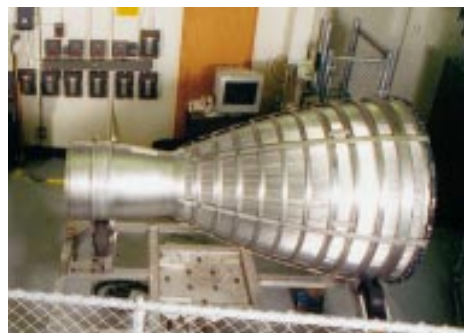
Figure 3-25: Side view of a regeneratively cooled nozzle.
