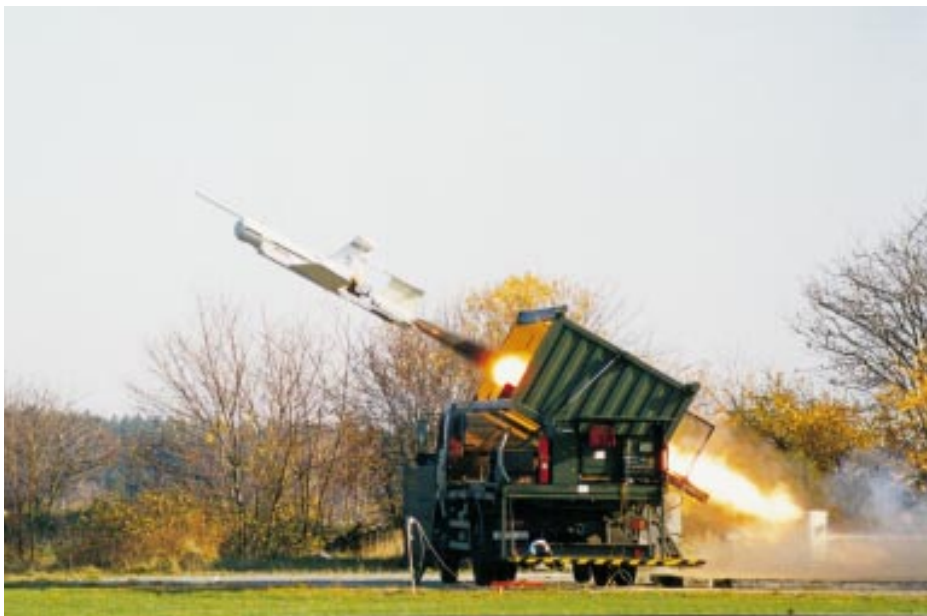
Figure 19-3: A propeller-driven UAV launched from a rocket booster.
