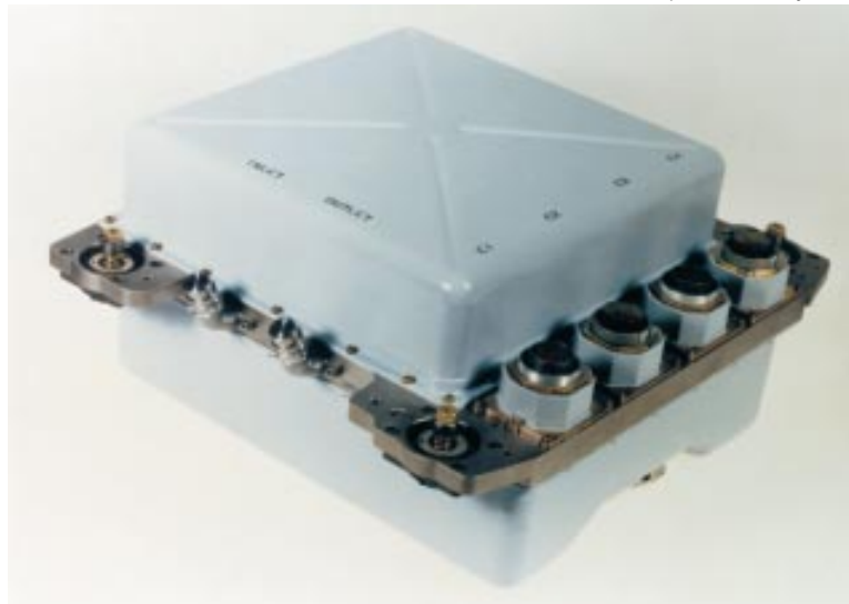
Figure 13-4: A radiation-hardened electronics assembly with liquid cooling.
