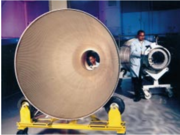
Figure 3-26: End views of regeneratively cooled nozzles.
