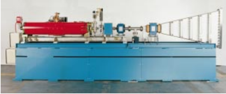
Figure 15-24: A 10 MeV X-ray machine used for sterilization (not MTCR-controlled).
