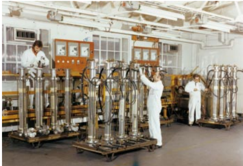
Figure 5-1: Tactical motors with cast-cure tooling attached.
