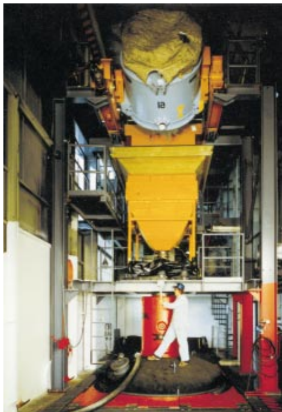
Figure 5-3: A propellant casting pit, with a motor case belowground.
