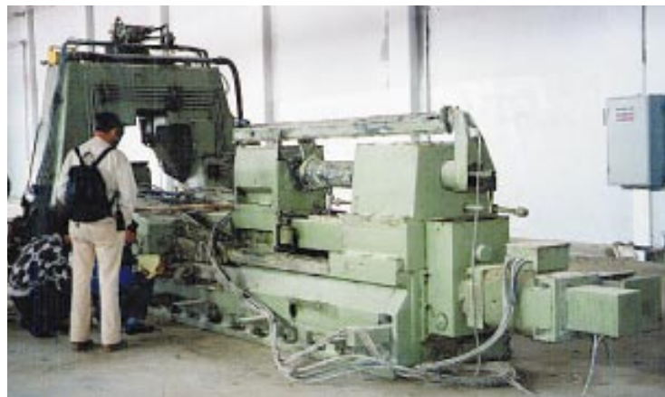
Figure 3-39: A horizontal flow-forming machine.
