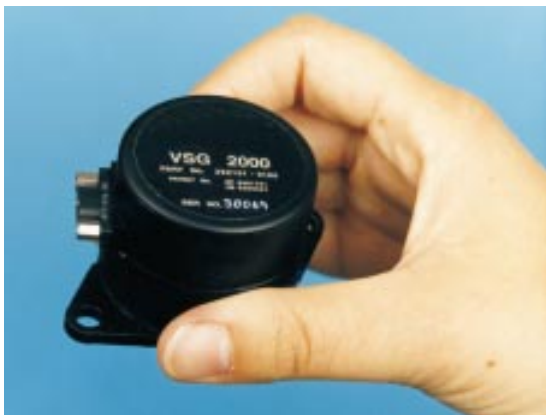
Figure 9-8: A vibrating structure gyro.
