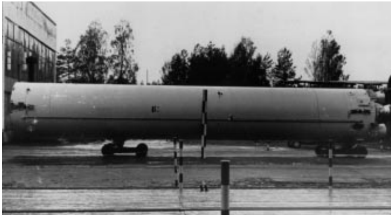
Figure 2-2: The first stage of a liquid-fueled ICBM.
