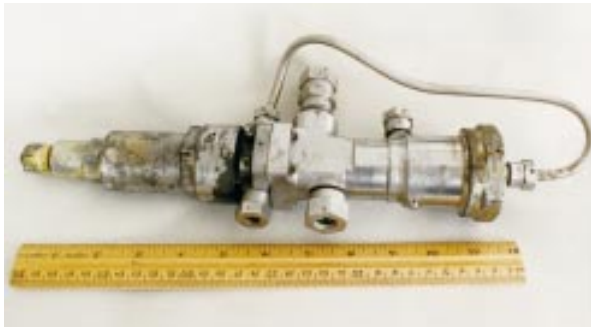
Figure 3-31: A servo valve from a Scud missile.
