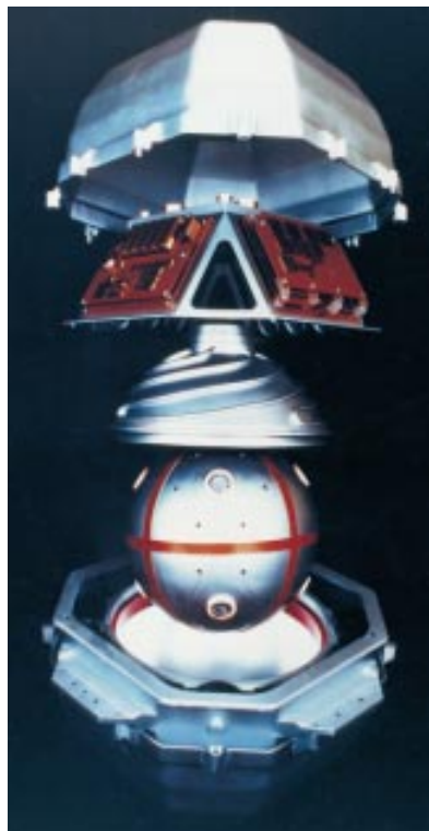
Figure 9-16: A strapdown IMU that contains three accelerometers and three ring laser gyros (in the end opposite the cables).
