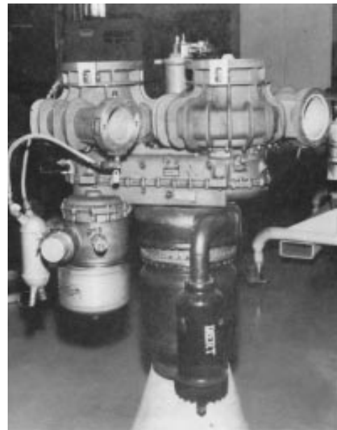
Figure 3-36: A multi-shaft turbopump assembly.
