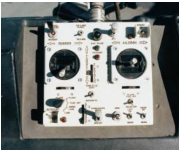
Figure 12-24: A portable flight controller console for an unmanned air vehicle.
