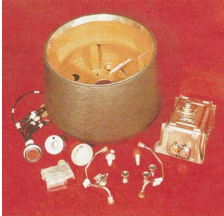
Figure 2-38: The aft end of an RV with the aft arming and fusing electronics box on the right.
