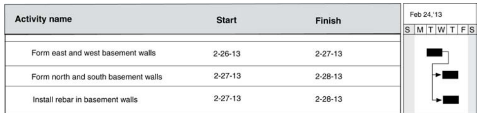
Figure 18: Eliminating Leads with Finish-to-Start Links
