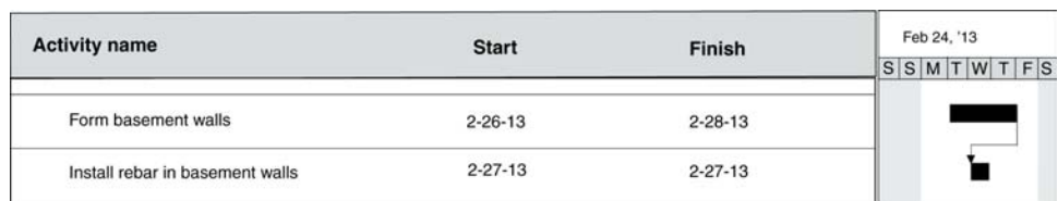
Figure 19: Logic Failure Associated with a Lead
