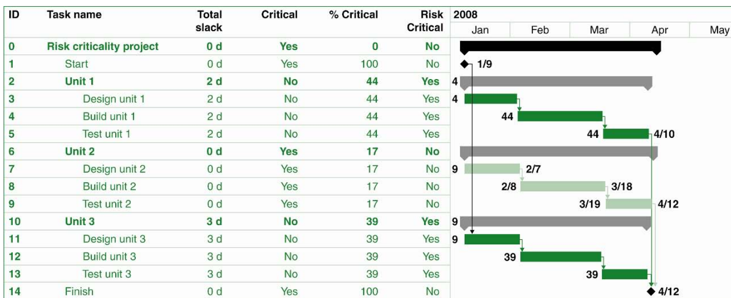
Figure 40: The Results of a Monte Carlo Simulation for a Schedule Showing a Critical Path
