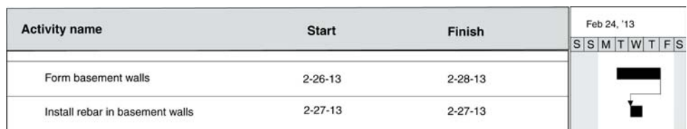
Figure 19: Logic Failure Associated with a Lead
