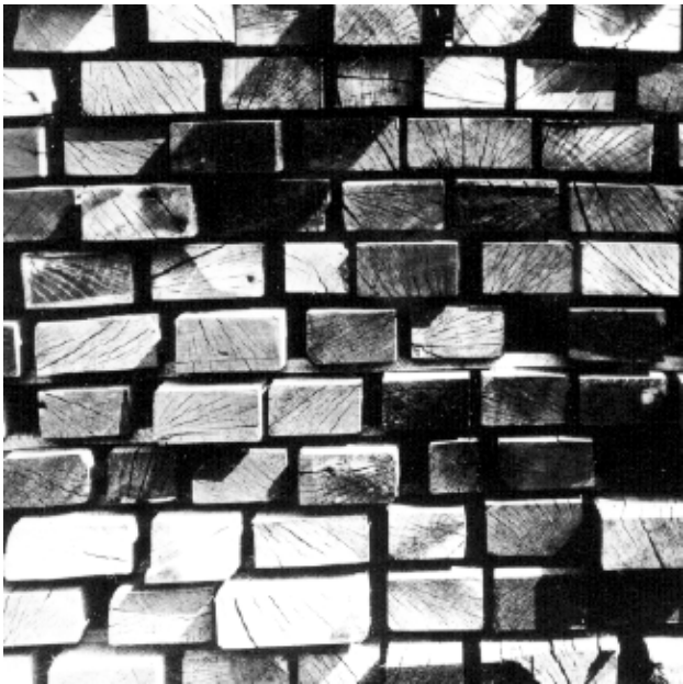
Figure 12-9. End checking in oak lumber.
