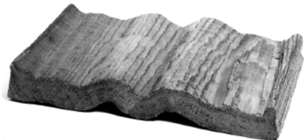
Figure 12-10. Severe collapse in western redcedar.
