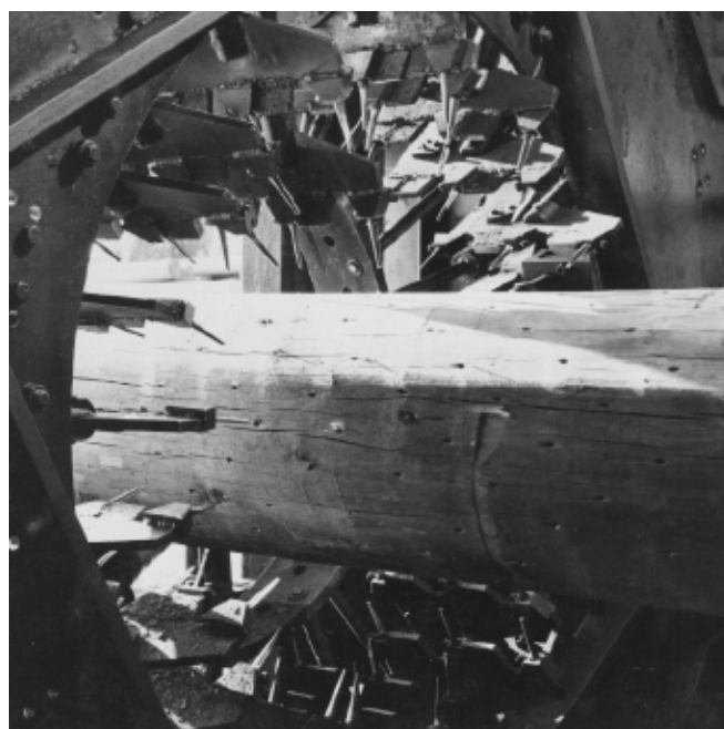
Figure 14-2. Deep incising permits better penetration of preservative.
