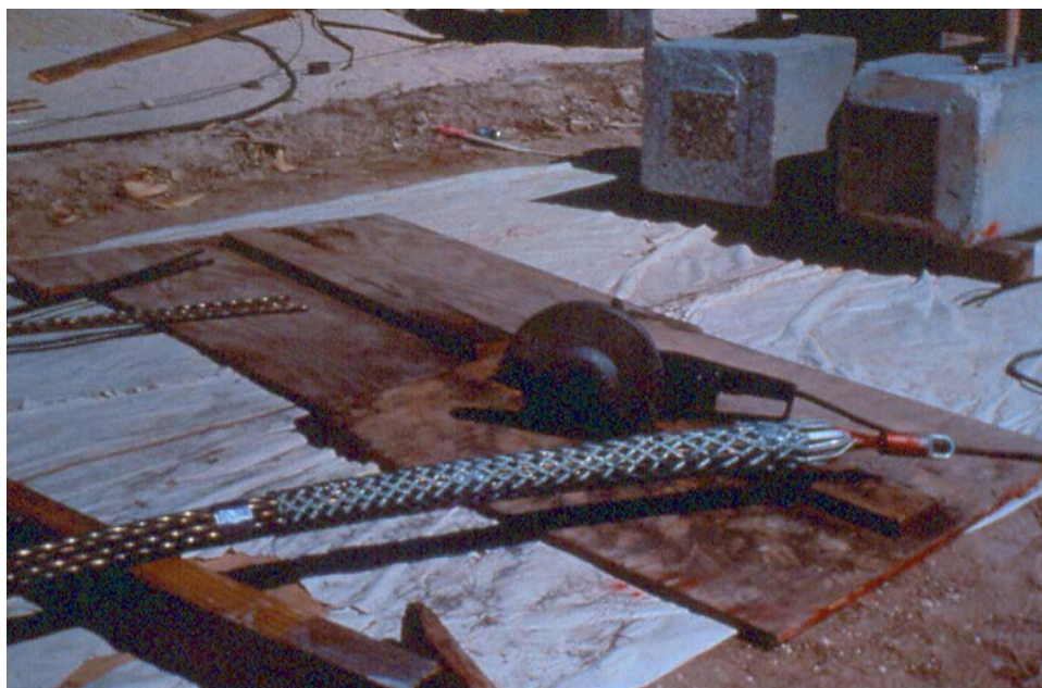
Figure 3.26 - Steel wire sock for installing multi-strand tendon
