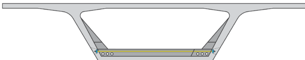
Figure 1.27 - Transverse Post-Tensioning in Deviator Ribs
