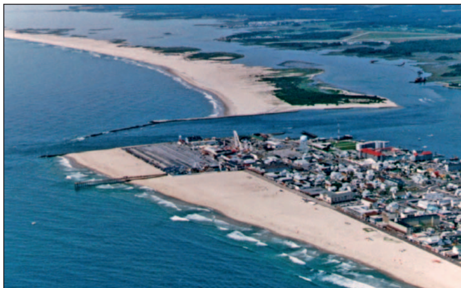
Figure 3-41. Ocean City Inlet, MD, was opened by a hurricane in 1933 and stabilized by jetties in 1934–35 that have resulted in extreme shoreline offset and downdrift erosion (1992 photograph)
