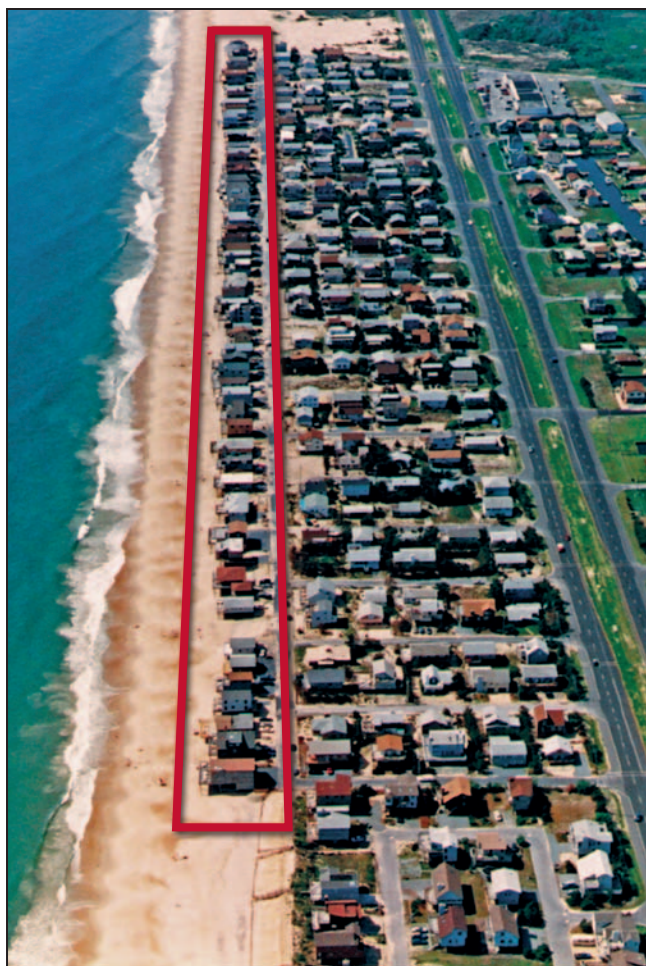
Figure 3-47. Long-term erosion at South Bethany Beach, DE, has lowered ground elevations beneath buildings and left them more vulnerable to storm damage
