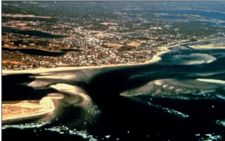
Figure 3-35. A January 1987 nor'easter cut a breach across Nauset Spit on Cape Cod, MA; the breach grew from an initial width of approximately 20 feet to over a mile within 2 years, exposing the previously sheltered shoreline of Chatham to ocean waves and erosion SOURCE: JIM O'CONNELL, USED WITH PERMISSION
