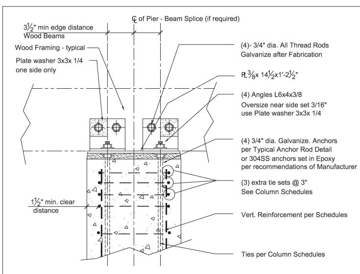
Double Angle Beam ( DAB ) - Typical Connection Section
