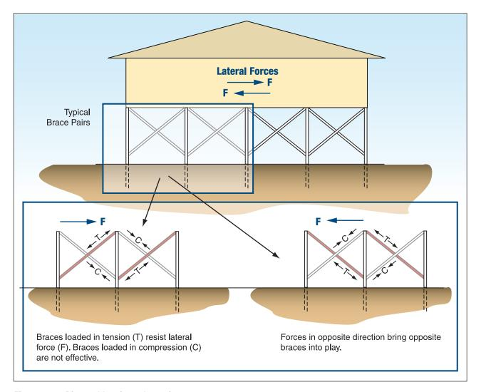
Figure 2-11. Diagonal bracing schematic.
