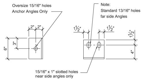
Double Angle Beam (DAB) - Typical Connection Section
