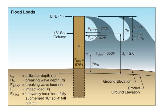
Table D-2. Loads on Columns Spaced 7 Feet On Center (for three rows of columns)
