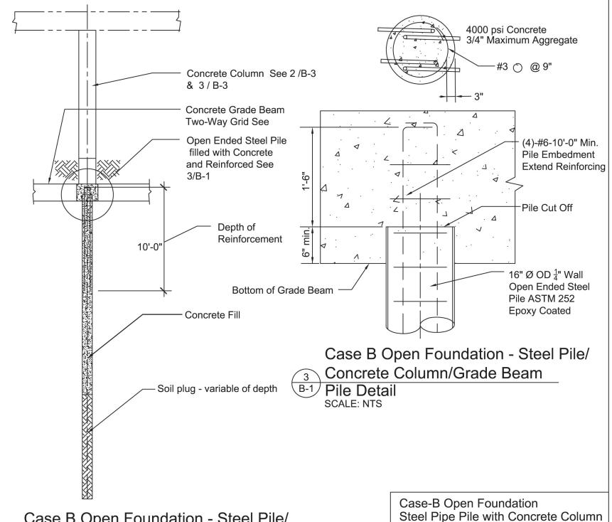
Case B Open Foundation - Steel Pile/ Concrete Column/Grade Beam
