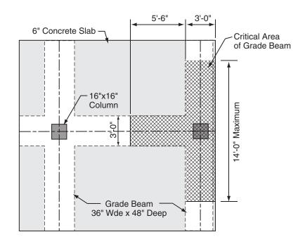
Figure D-7. Loading Diagram for Open Foundation Example.
