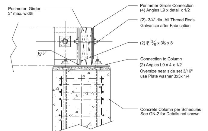
Captive-Clamped Beam ( CCB ) - Typical Corner Connection Section
