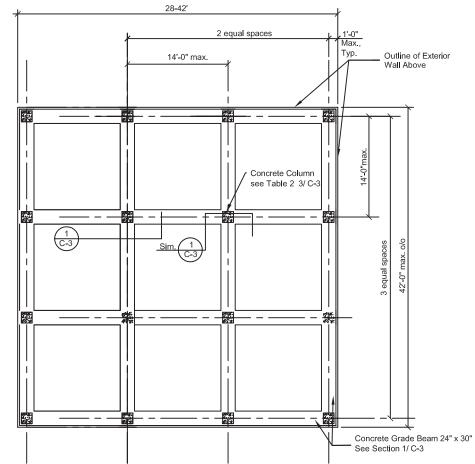
6 - Bay Foundation Column and Beam Plan
