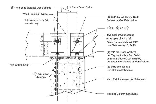
Captive-Clamped Beam (CCB) - Typical Connection Elevation GN-2 SCALE: NTS
