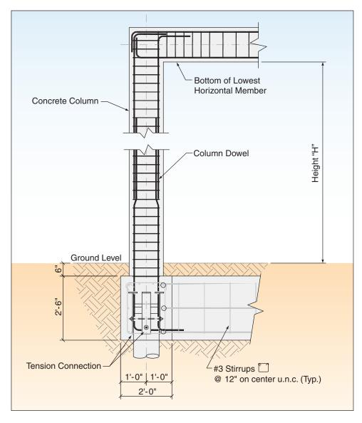
Sections were designed with an emphasis on strength, ductility, and constructability. To simplify detailing and construction, axial and shear reinforcement were made consistent through each section. Section properties throughout each member were selected to resist the maximum forces (positive and negative moments, axial loads, and shears) that exist within the elements (grade beams, columns, or elevated beams). To simplify forming, the dimensions of the
