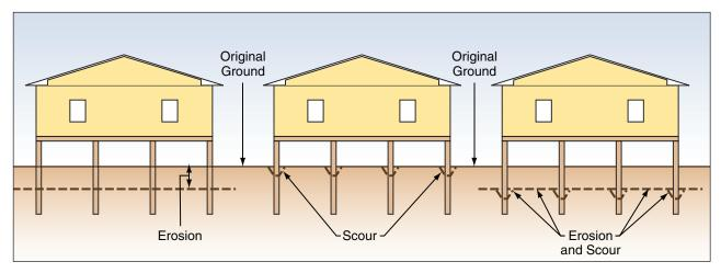
Figure 3-5. Distinguishing between coastal erosion and scour. A building may be subject to either or both, depending on the building location, soil characteristics, and flood conditions.
