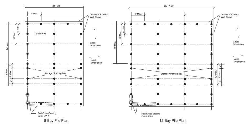
Case A Open Foundation - Driven Treated Timber Pile Pile Plan - 1 SCALE: NTS
