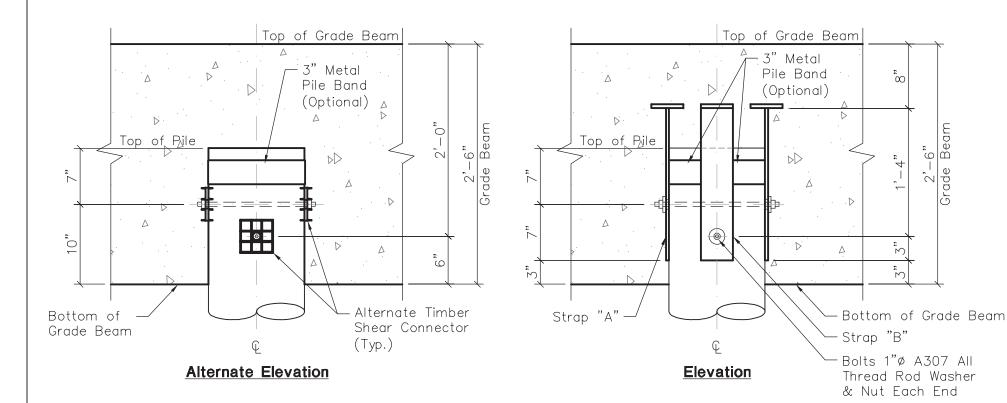
Pile To Grade Beam Tension Connection Details
