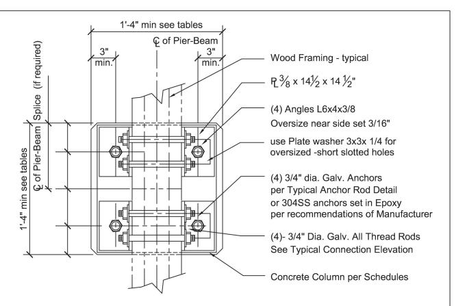
Double Angle Beam ( DAB ) - Typical Connection Plan Detail
