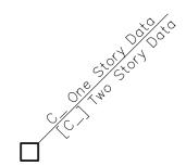
Information Displayed Above The Tag Line Is To Be Used For One Story Design, Information Displayed Below The Tag Line, Contained In [] Square Brackets, Is To Be Used For Two Story Design.
