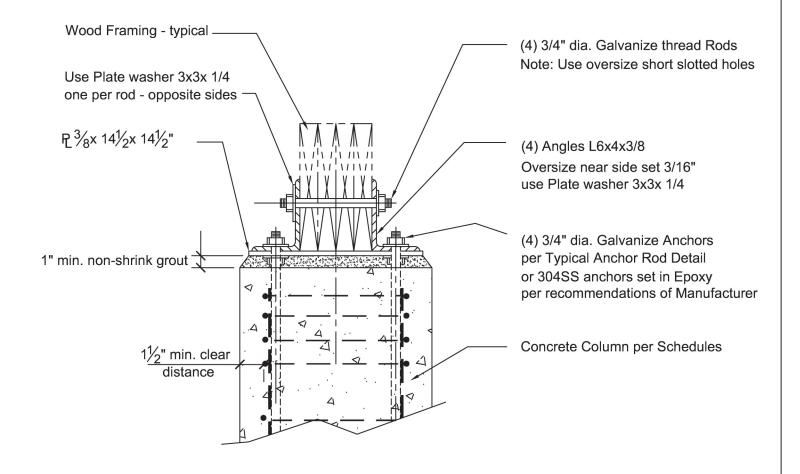
Double Angle Beam ( DAB ) - Typical Connection Section
