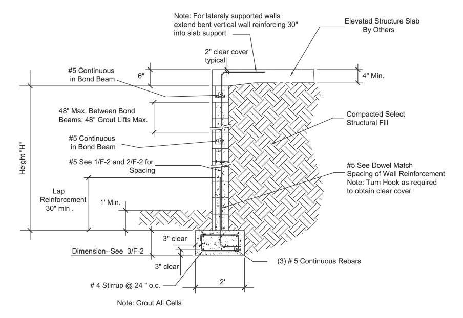
Case F - Closed Foundation Reinforced Masonry Foundation - Stem Wall
