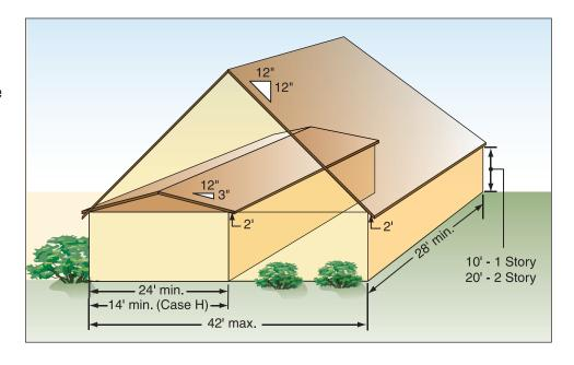
and roof pitches. Appendix C contains a complete list of criteria and assumptions used in these designs.
