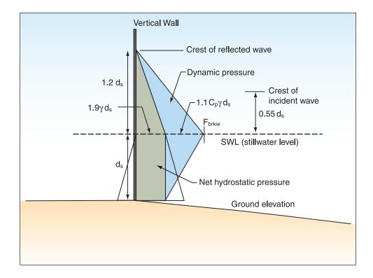
For the sample calculations, Case 1 was used (see Figure D-5) with a breaking wave load of 623 pounds applied to a non-critical column. The loads were then determined and summarized. Since the calculations must combine distributed loads on the elevated structure and discrete loads on the columns themselves, a column spacing of 7 feet is assumed in the calculations. For lateral loads on the structure, calculations are based on three rows of columns sharing lateral loads (Table D-2).
