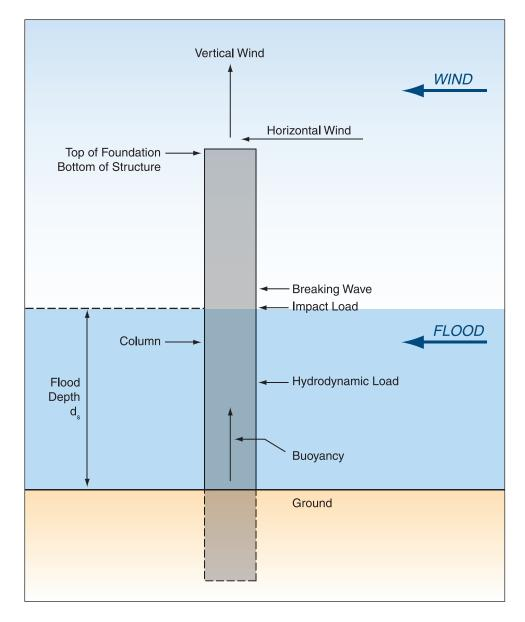
Loads on the foundation elements themselves are more difficult to tabulate because they depend on the foundation style (open or enclosed), foundation dimensions, and foundation height. Table 4-2 provides reactions for the 18-inch square columns used in most of the open foundation designs.
