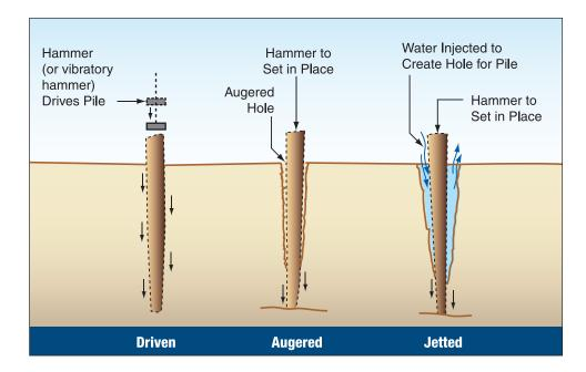
If steel piles are used, only the hammer driving method mentioned above should be used. For any pile driving, the authority having jurisdiction or the engineer-of-record may require that a driving log is kept for each pile. The log will tabulate the number of blows per foot as the driving progresses. This log is a key factor used in determining the pile capacity.
