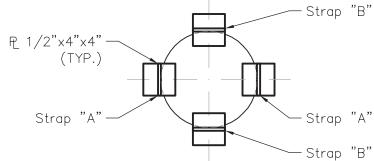
Timber Shear Connector & Pile Top View
