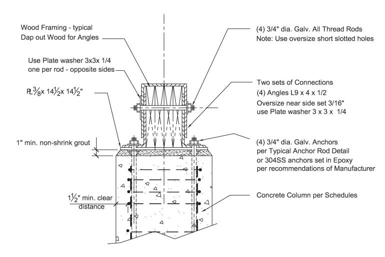
Captive-Clamped Beam ( CCB ) - Typical Connection Section Scale: NTS
