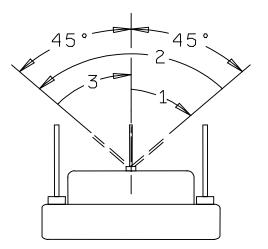
FIGURE 3 Wire-lead bend test.
