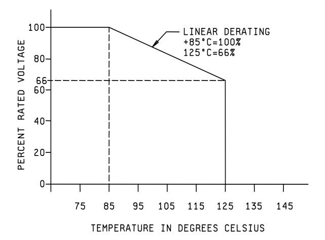
FIGURE 2. Voltage derating with temperature.
