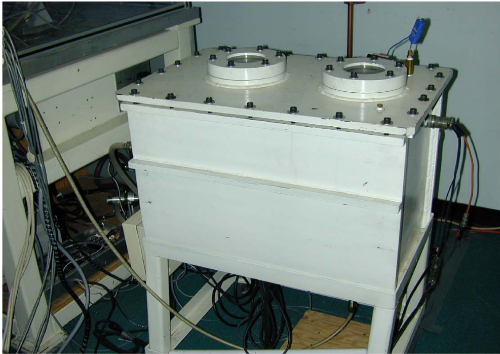
Figure 3. Pressurized Screw-Feeder Sand Plenum.
