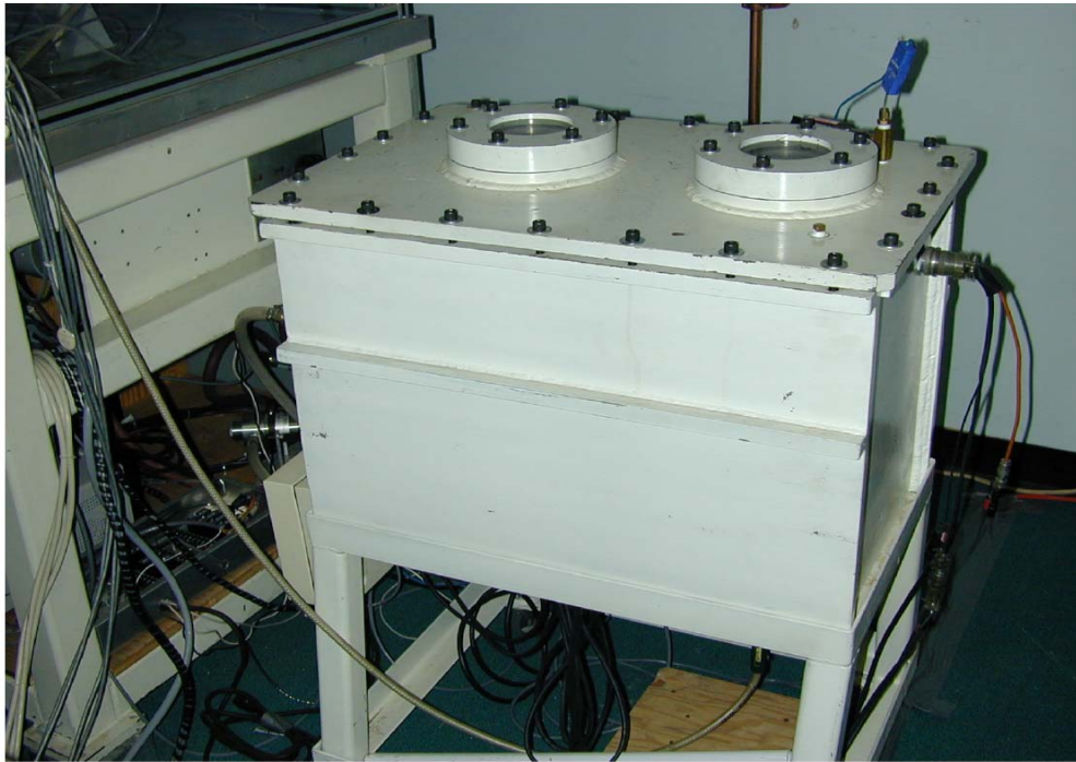
Figure 3. Pressurized Screw-Feeder Sand Plenum.
