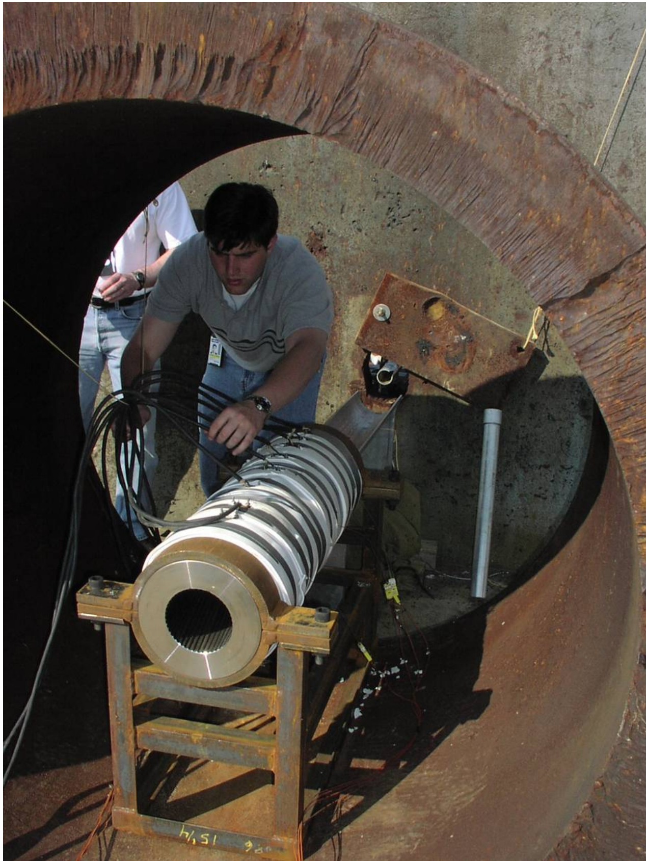
FIGURE 2. Gun simulator test fixture (projectile tests).
