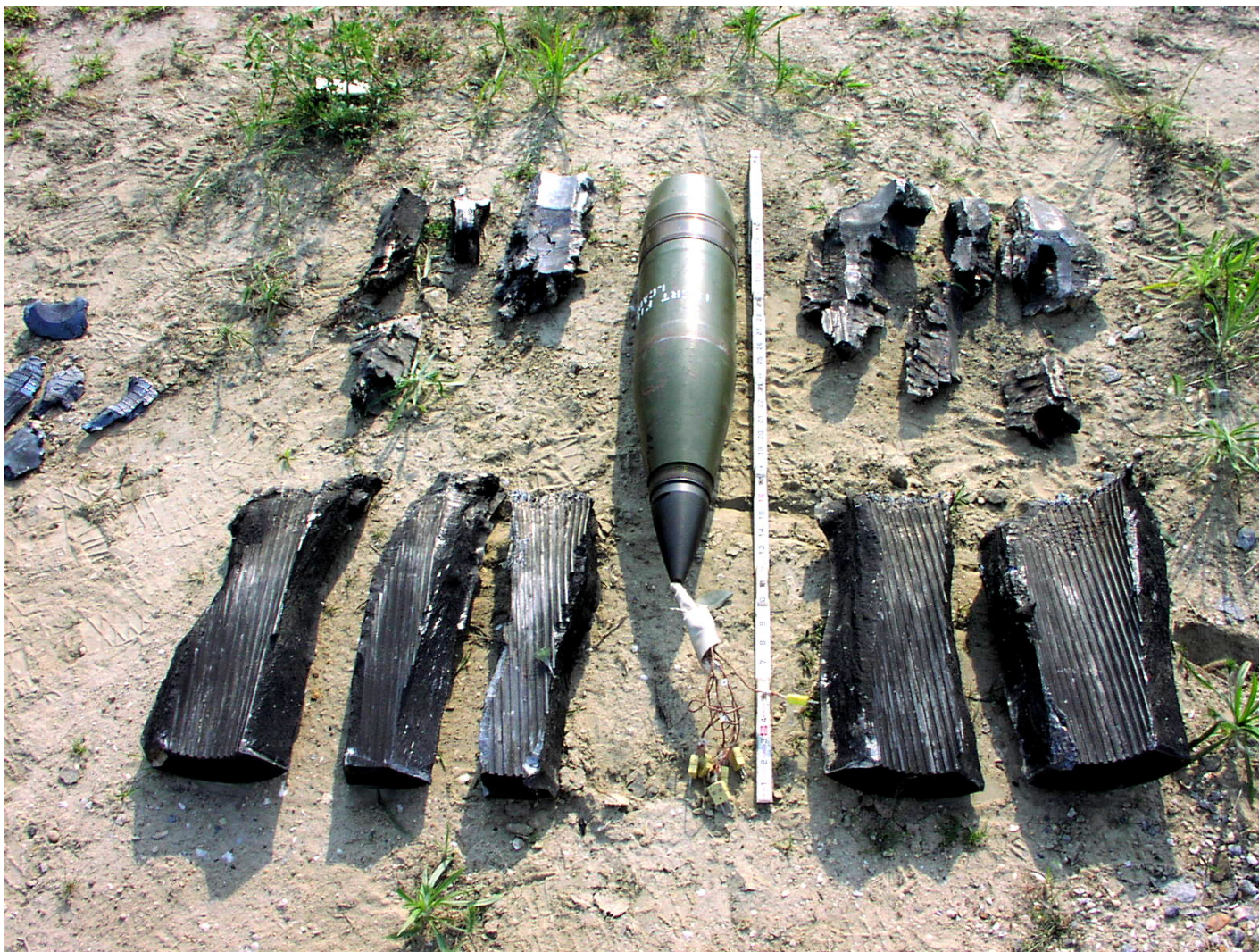
FIGURE 6. Example of barrel fragments produced by a projectile cook-off reaction.
