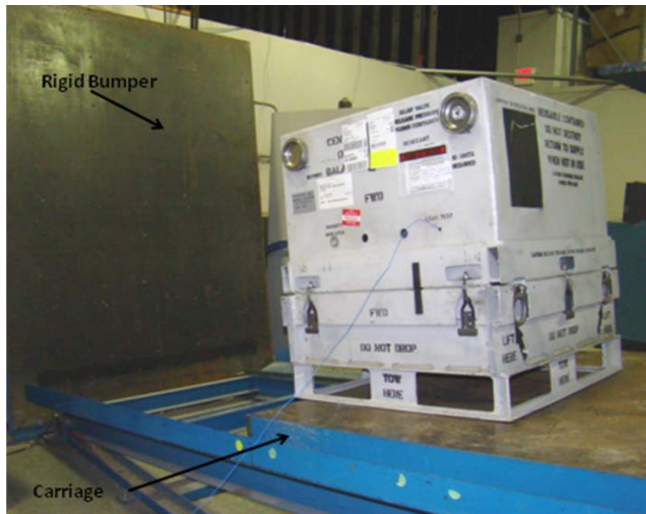
FIGURE 20. Incline impact test setup.
