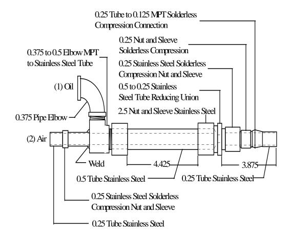
FIGURE A2. Fabrication details for oil spray atomizing nozzle.
