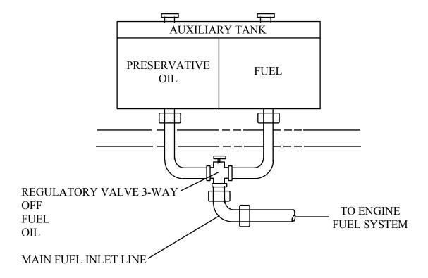
FIGURE 4. Auxiliary fuel container.
