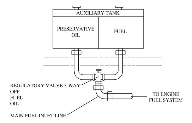
FIGURE 4. Auxiliary fuel container.
