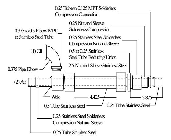
FIGURE 2. Fabrication details for oil spray atomizing nozzle.
