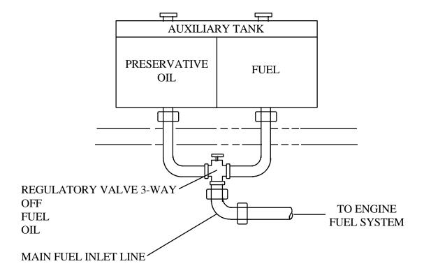
FIGURE 4. Auxiliary fuel container.
