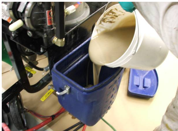
FIGURE A-5. Charging the reaction spray equipment with the components.
