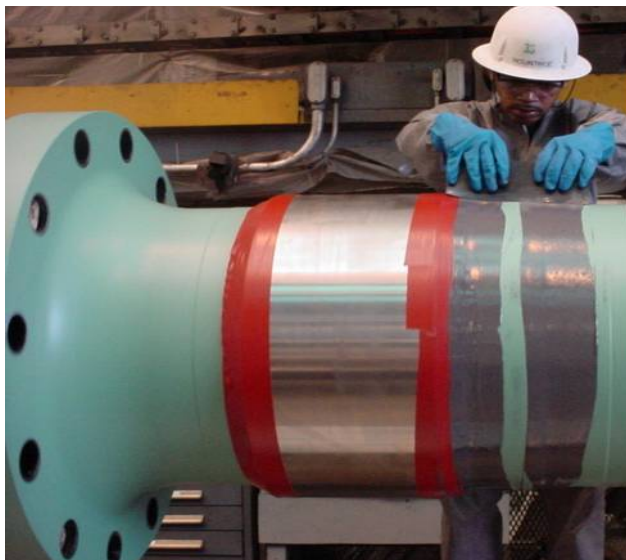
FIGURE A-11. Fairing the shaft/sleeve interface with sealing/fairing compound.
