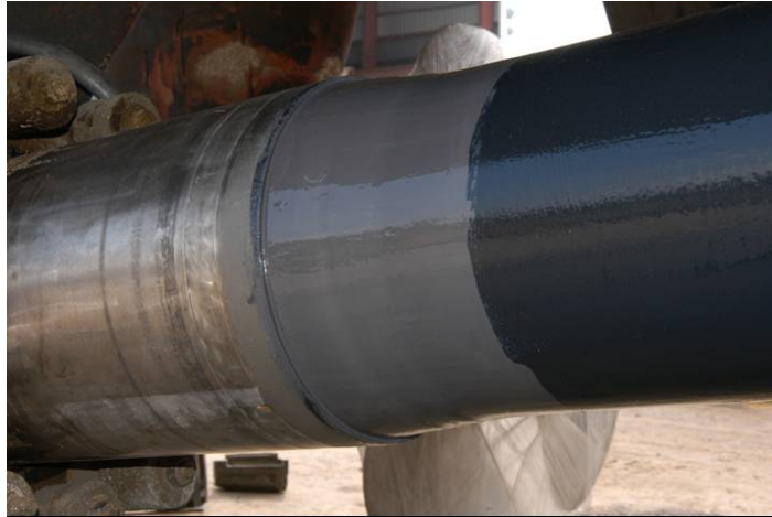
FIGURE A-13. View of gray sealing/fairing compound applied over second layer of elastomeric coating (black).
