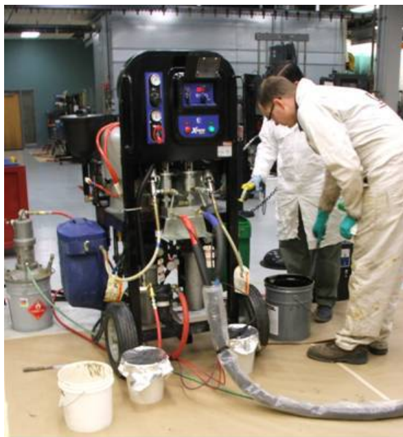
FIGURE A-3. Plural component reaction spray equipment.
