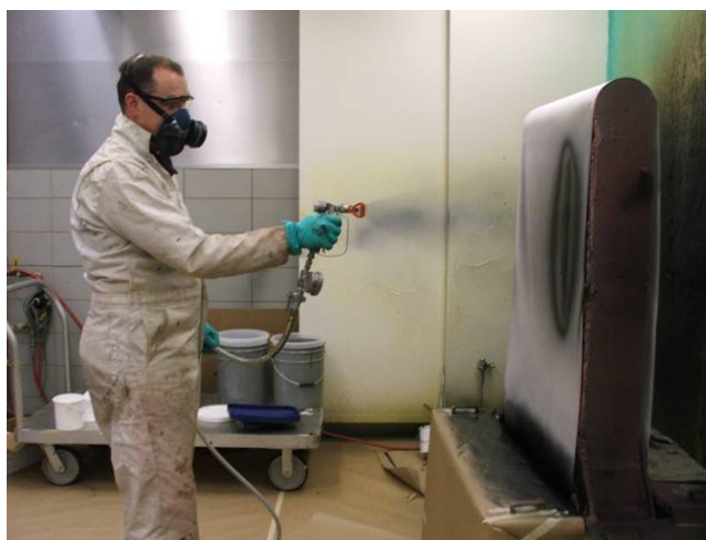
FIGURE A-7. Reaction spray of elastomeric coating.
