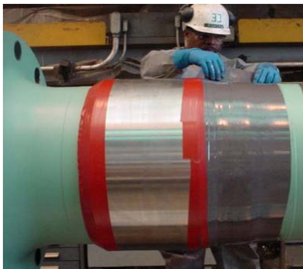
FIGURE A-12. Completion of shaft-to-sleeve fairing with sealing/fairing compound.
