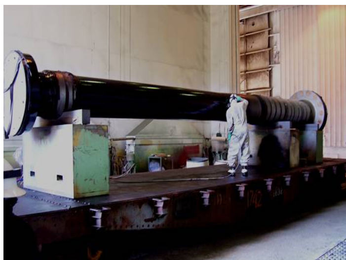
FIGURE A-6. Application of elastomeric coating by reaction spray at a shipyard.
