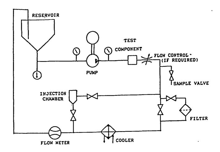
FIGURE 1. Contamination sensitivity test circuit.
