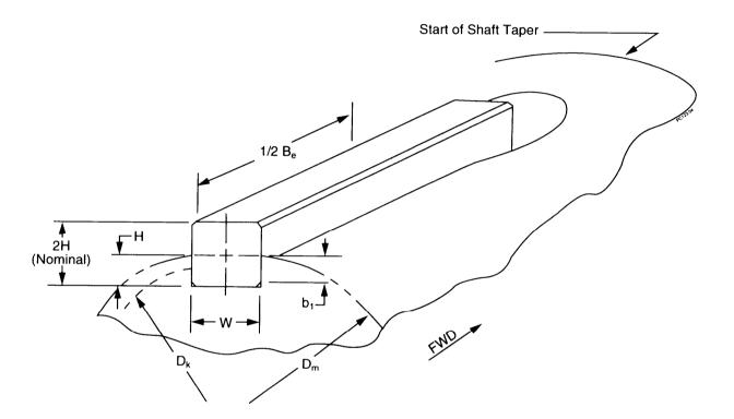
Figure 4. Propeller Key
